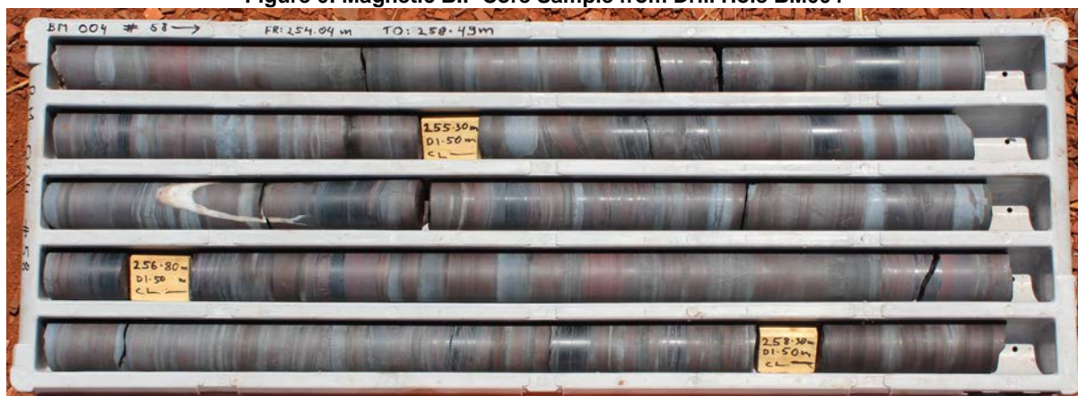
Figure 6: Magnetic BIF Core Sample from Drill Hole BM004
