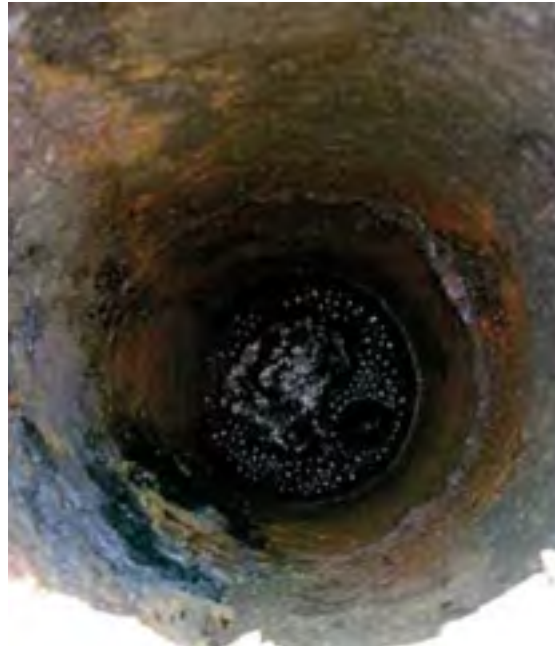
Figure 5 - Coal exploration drill hole with gas bubble visible at the standing water table a few metres below surface.
