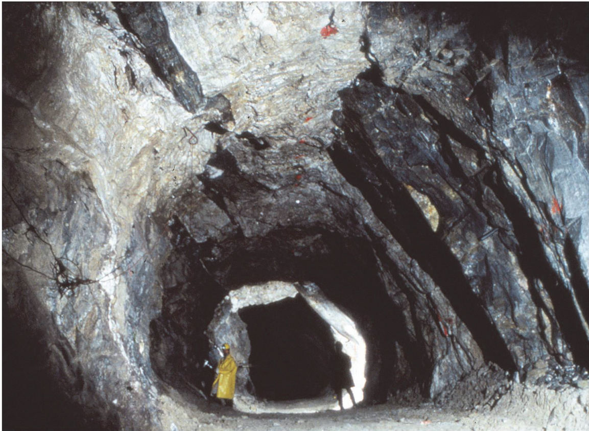
Photo 1: Underground drive along a Pegmatite dyke which contains Spodumene the lithium mineral.
