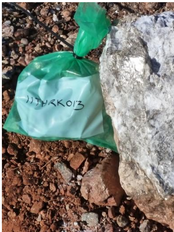
Figure 1: Soil & rockchip sampling of pegmatites
