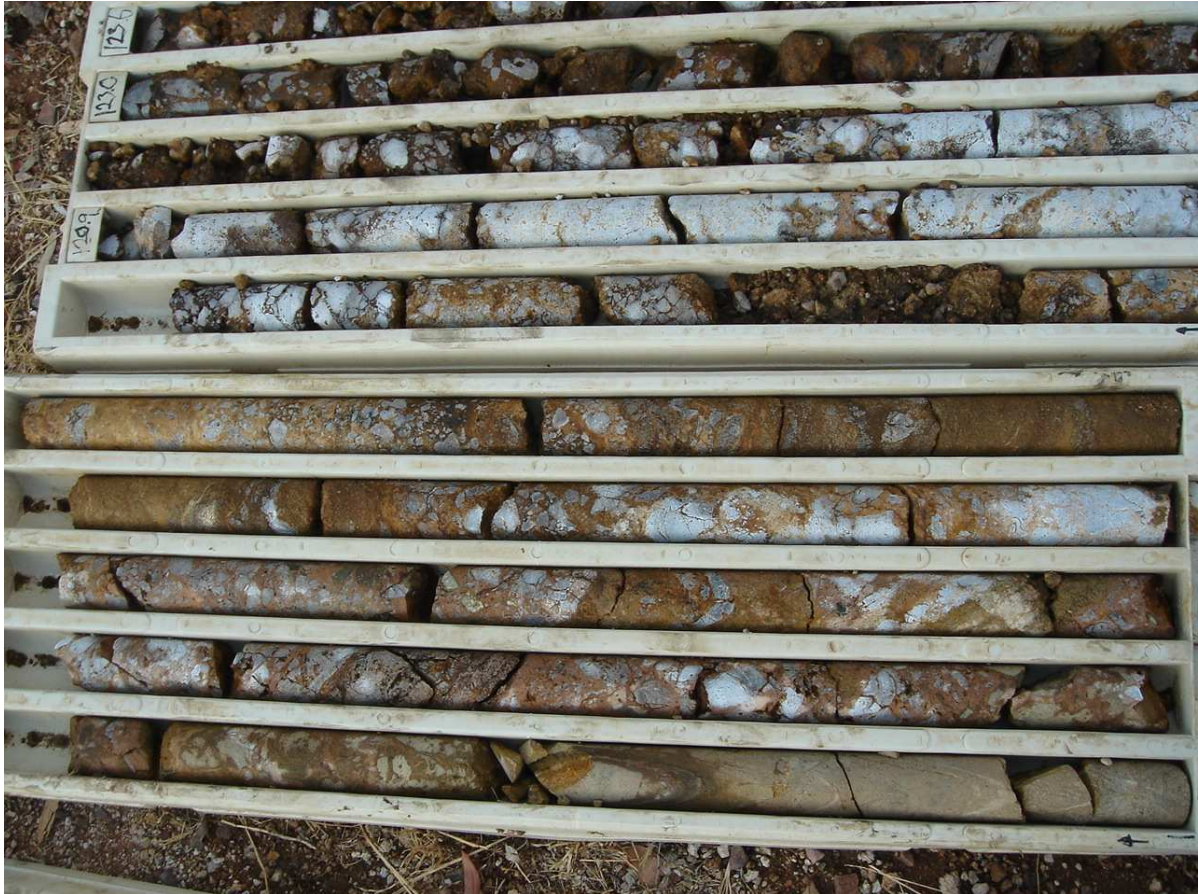
Photograph 1: Wide zones of iron oxide breccia intersected over 30 meters in drill hole MC09DD02 at QMC's Morris Creek Prospect.
