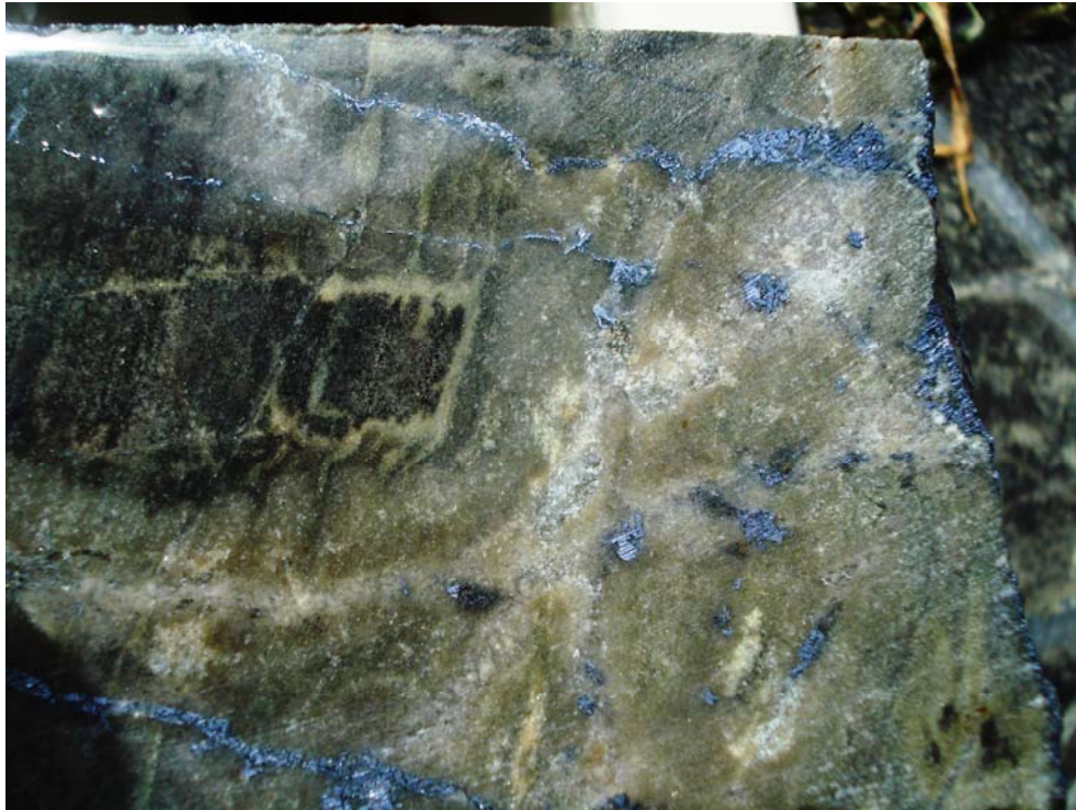
Molybdenite in altered schist, Hole RCD13, 260.5m depth. This hole assayed 2,930 ppm Mo from 260-262m
