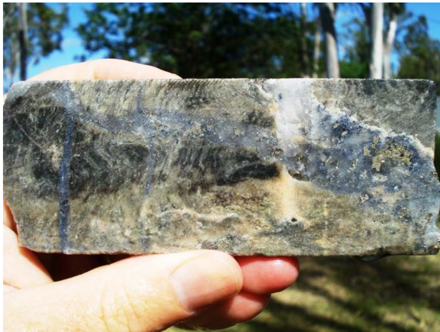
Quartz-pyrite-molybdenite vein in altered schist. Hole RCD31, 197.9m depth. Drill core not yet assayed
