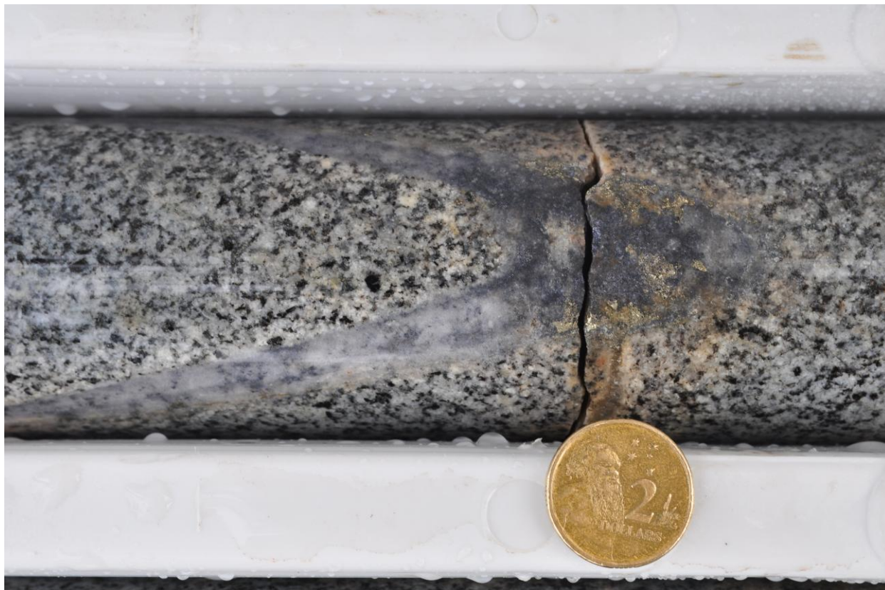
RCD 55 at 686.95m. Fine grained, disseminated molybdenite and pyrite in fine crystalline quartz vein (host rock monzonite)
