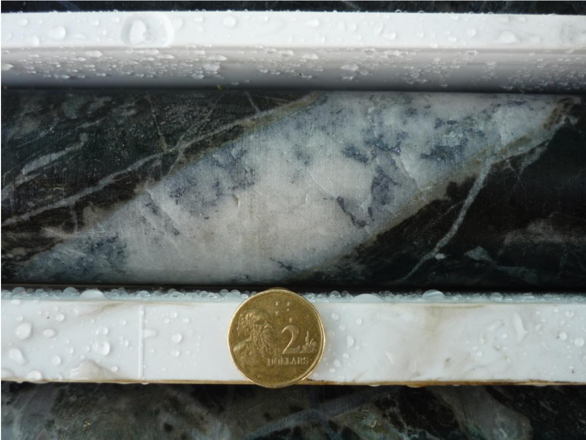
RCD 56 at 422m. Quartz-molybdenite vein featuring sericite-pyrite vein-selvage alteration within biotite-hornfels
