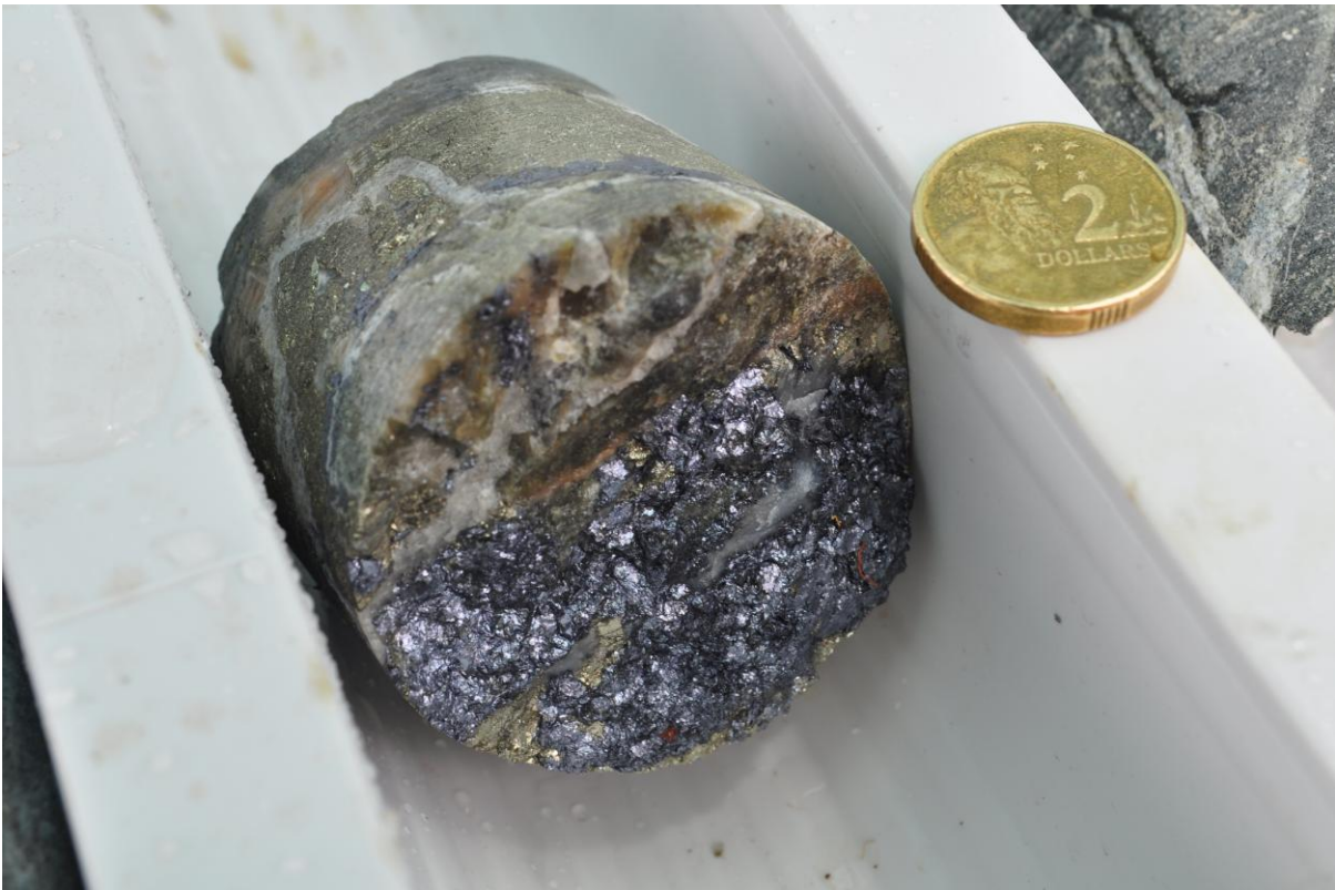
RCD 56 at 625.4m. Coarse grained molybdenite vein cutting across multiple phases of quartz and pyrite veining
