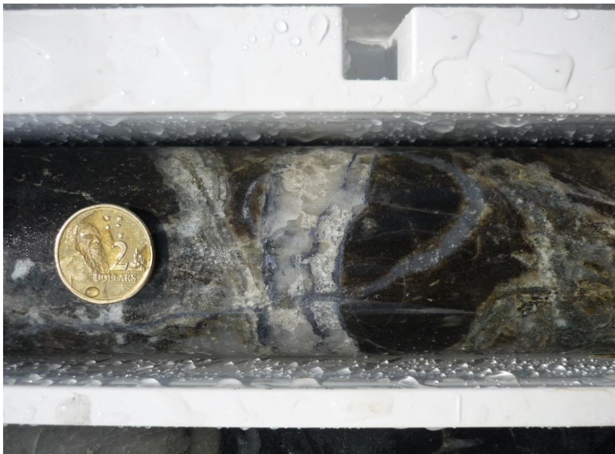
RCD 56 at 347m. Quartz-sericite-molybdenite-pyrite veins featuring sericite vein-selvage alteration within biotite-hornfels.
