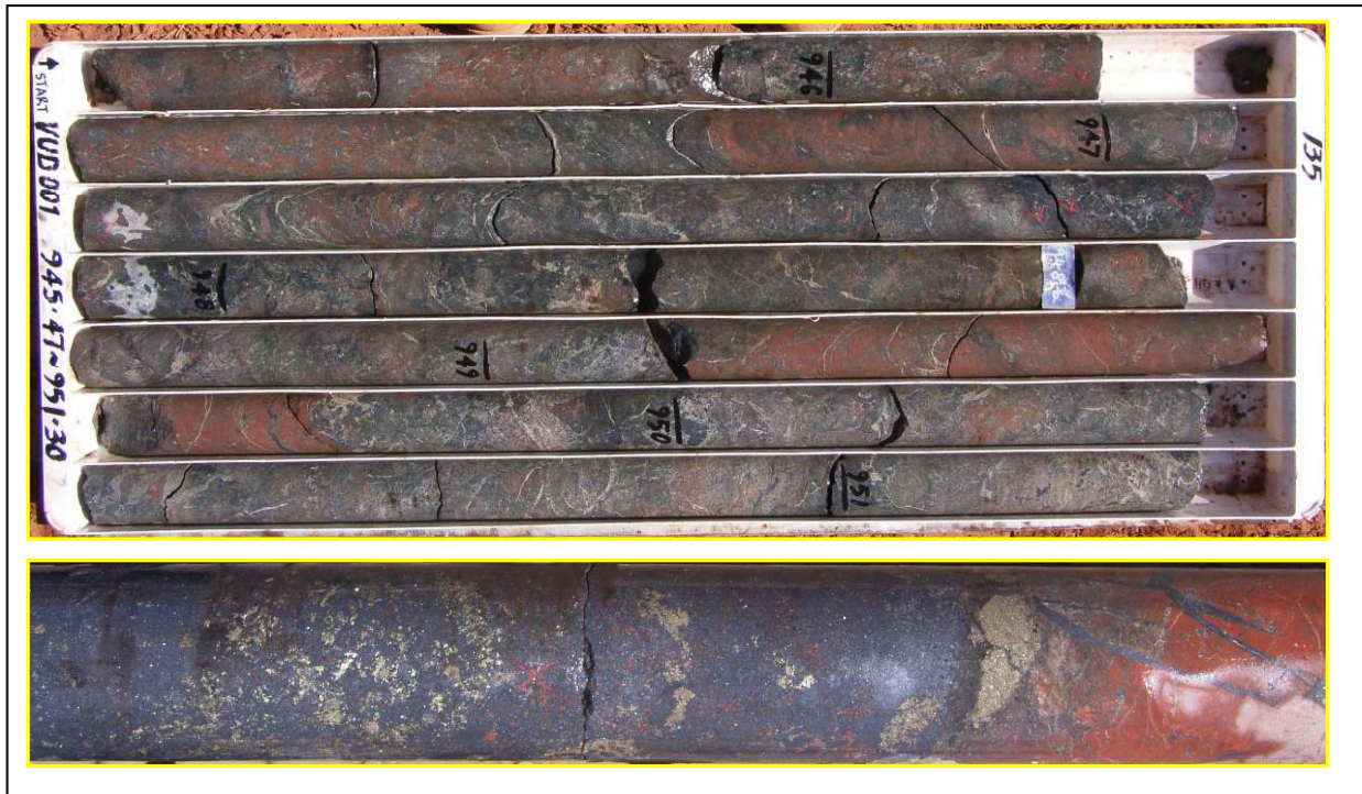
Figure 3: Upper photo: NQ size diamond drill core from VUD 001, showing hematite, carbonate (sericite, chlorite, sulphide alteration). Lower photo: Close-up of zone of strong hematite breccia development within (red) altered volcanic rocks.
