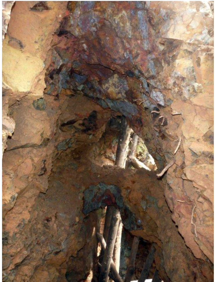
Sub-vertical zone of silica-magnetite-sulphide mineralisation
