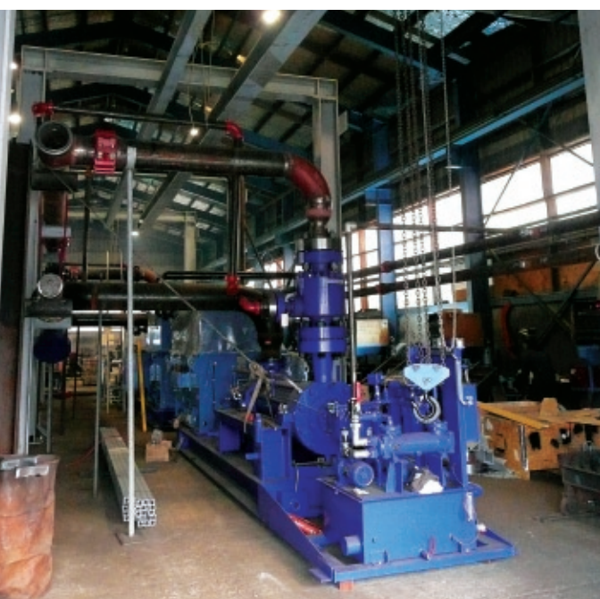
Hydro monitor pump station being assembled for testing before being deployed underground
