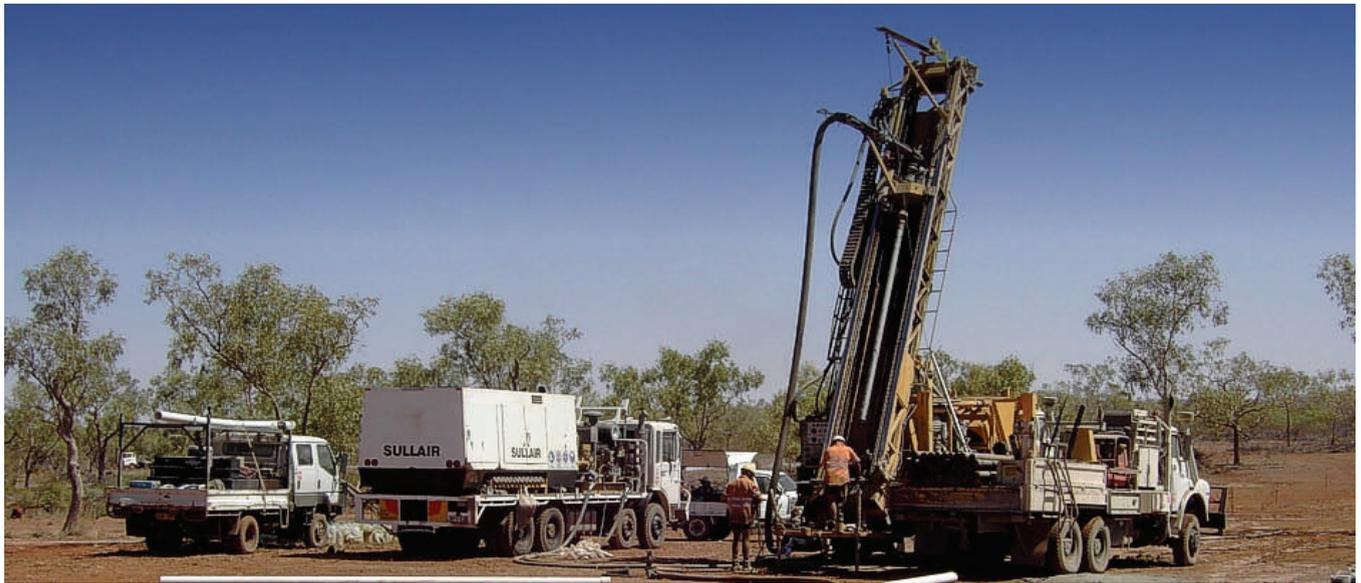
Fig 22: RC rig drilling at Rainden
