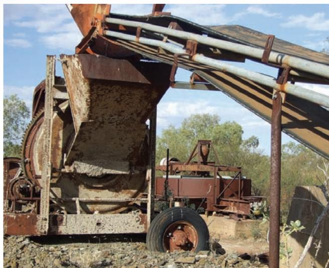
*Fig 3: Historic equipment left behind at the old Double Oxide Mine; feed conveyor to large cement mixer style tumbling unit, which was used to separate native copper from the fresh rock that was crushed in the grinding rolls drum in the background..*
