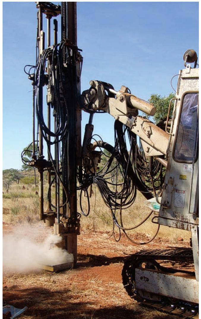
*Fig 27: RAB drill - Rock chips are sampled every metre down-hole. Each hole ends once it has drilled through approximately 1m of hard fresh bedrock, which is typically encountered at depths between 2 to 11 metres at Rocklands.*
