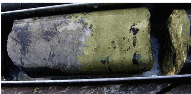
Fig 31: Diamond drill core showing the copper mineral chalcopyrite (yellow) and pyrite (mid grey). Cobalt is principally associated with pyrite at Rocklands.
