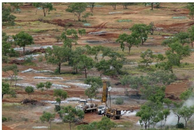
Fig 8: RC rig in a field of sample bags from previous drilling.
