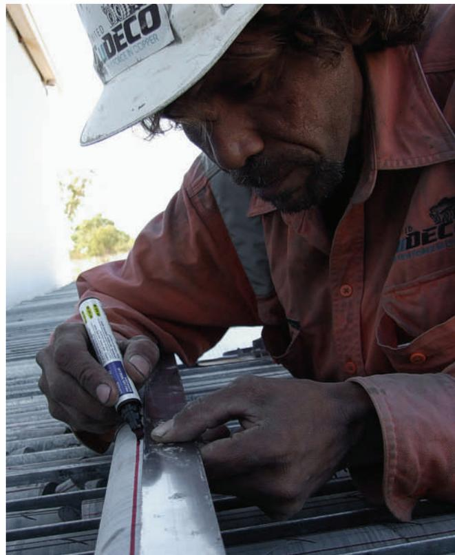
Fig 25: Guidelines being drawn on to solid diamond core in preparation for diamond cutting and prep for assay.
