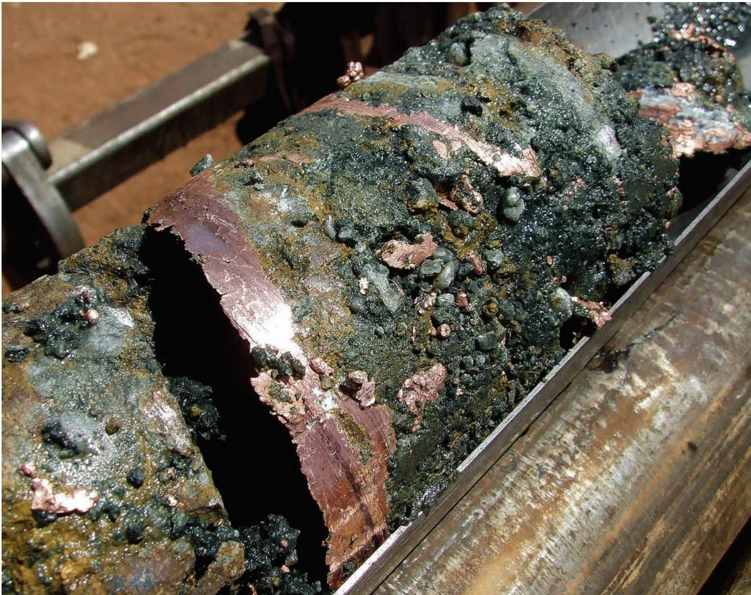
*Fig 10: Wide diameter PQ (85mm) metallurgical diamond core as it is retrieved from the drill string. Massive solid copper metal and chalcocite can be seen throughout. (Native copper contains 99.8% copper metal and chalcocite contains 79.85% copper metal).*
