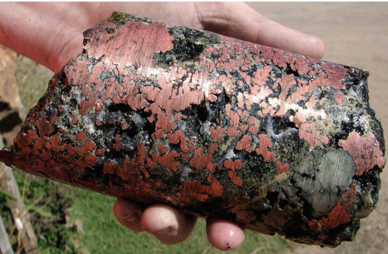
Fig 9: solid native copper in PQ (85mm), metallurgical diamond drill core.
