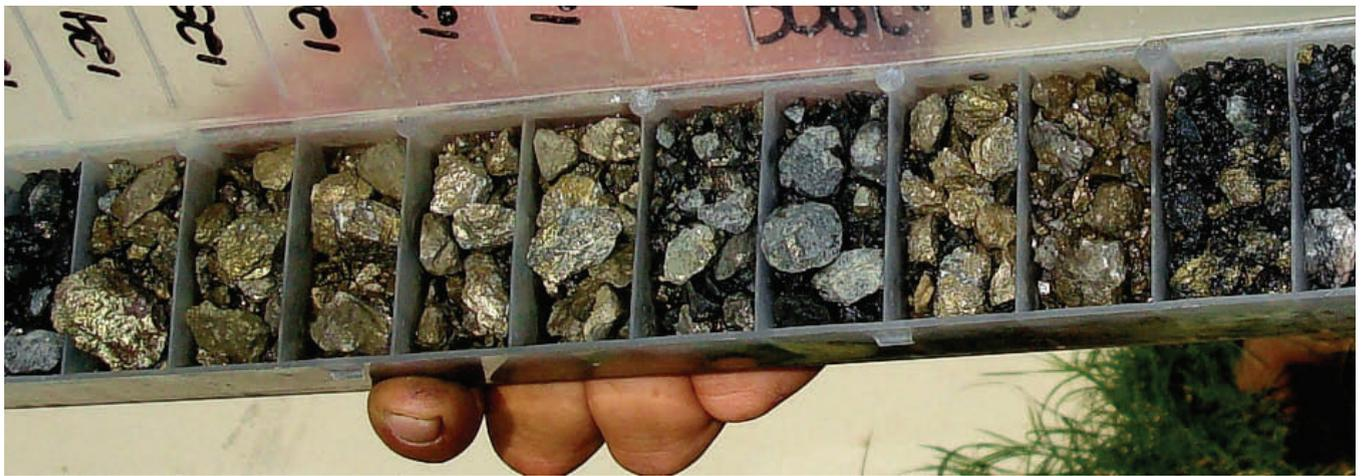
Fig 30: Cobalt is typically associated with pyrite at Rocklands. Shown above is chalcopyrite (high grade copper mineral), with associated pyrite.
