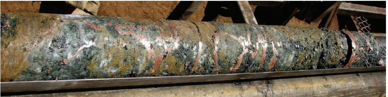
*Fig 11: Approximately 1.2m length of wide-diameter PQ (85mm) metallurgical diamond core DODH073, as it is retrieved from the drill string. Massive solid copper metal and chalcocite can be seen throughout. (Native copper contains 99.8% copper metal and chalcocite contains 79.85% copper metal).*
