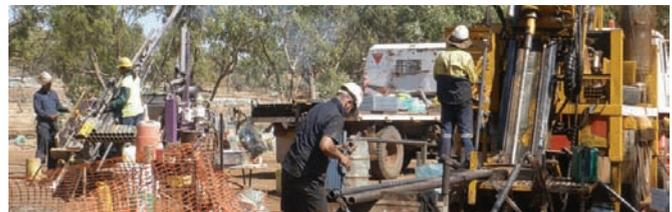
Fig 17: Metallurgical and structure targeted holes being drilled in central Las Minerale.
