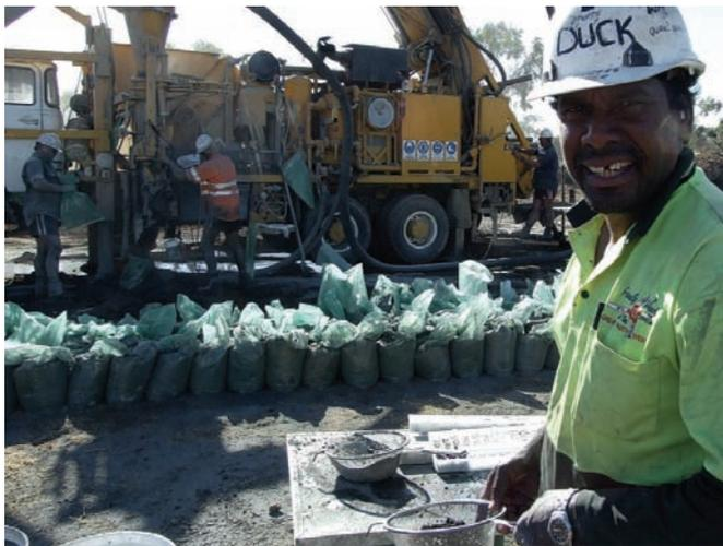
Fig 19: RC rig with drilling crew and field assistant preparing chip sample trays.
