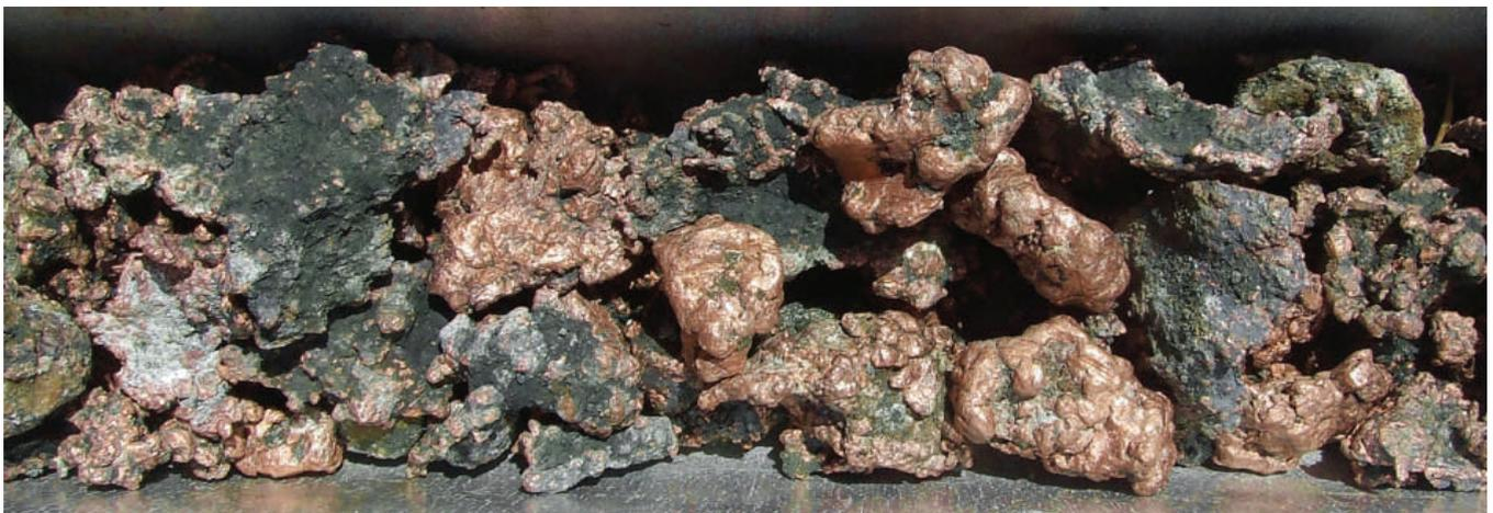
Fig 5: Solid native copper nuggets as straight from the PQ metallurgical diamond drill core.
