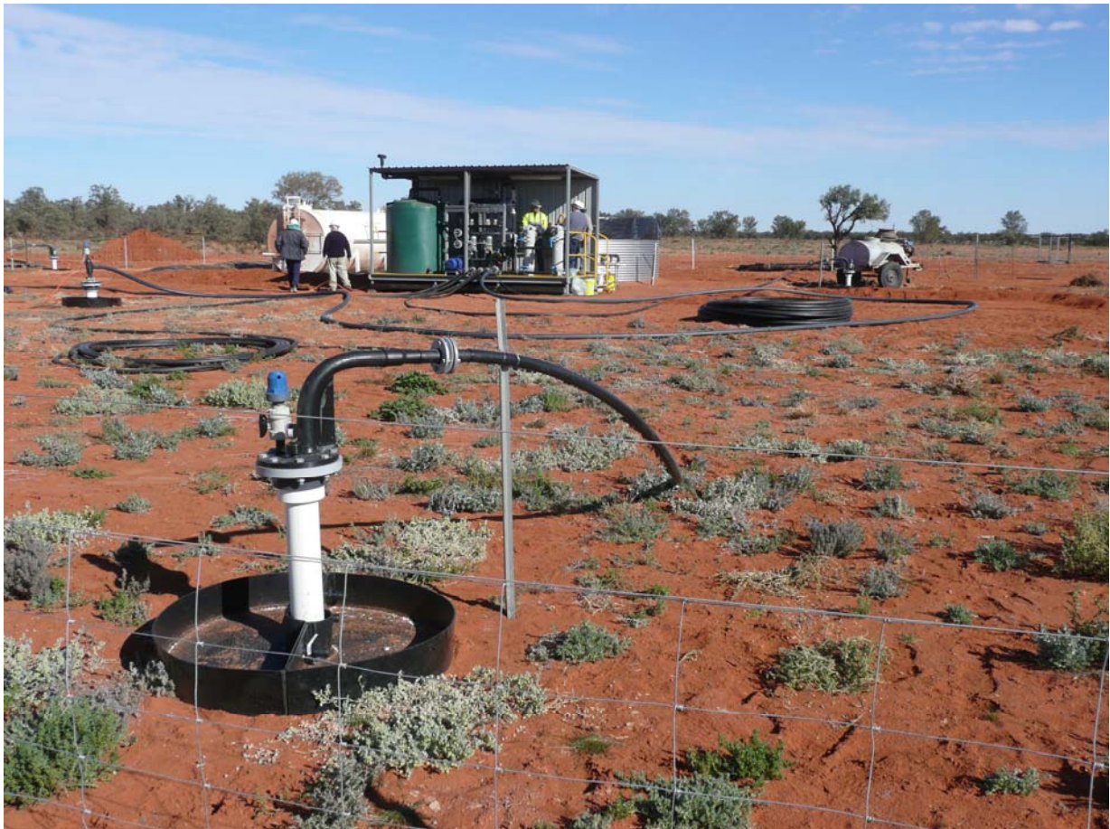
Figure 1: Well house unit in operation at Oban, showing pipe connections to injection well (foreground) and central extraction well (background and to left). All pipe work and connectors are specially designed and manufactured to high standards in order to avoid failure and leakage
