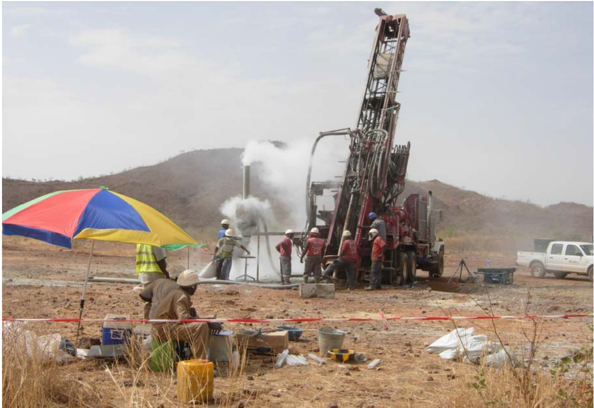
RC drilling on the SEMAPOUN prospect.
