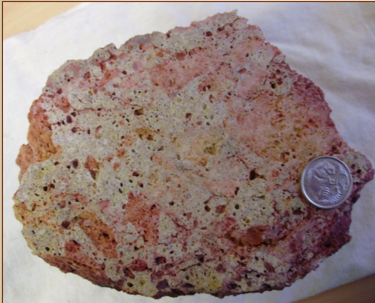
Leached, silicified and mineralised lapilli tuff
