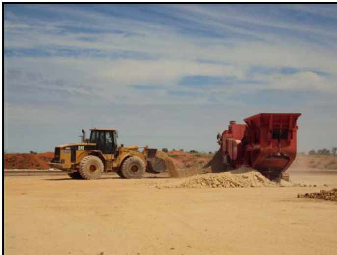
Crushing of Bulk Sample Material On-site – April 2010
