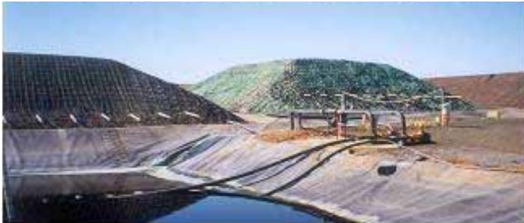
Figure 1. Bio-leach test of low-grade nickel sulphide of Jinchuan (13 th Goldman Sachs Basic Material Conference, New York)
