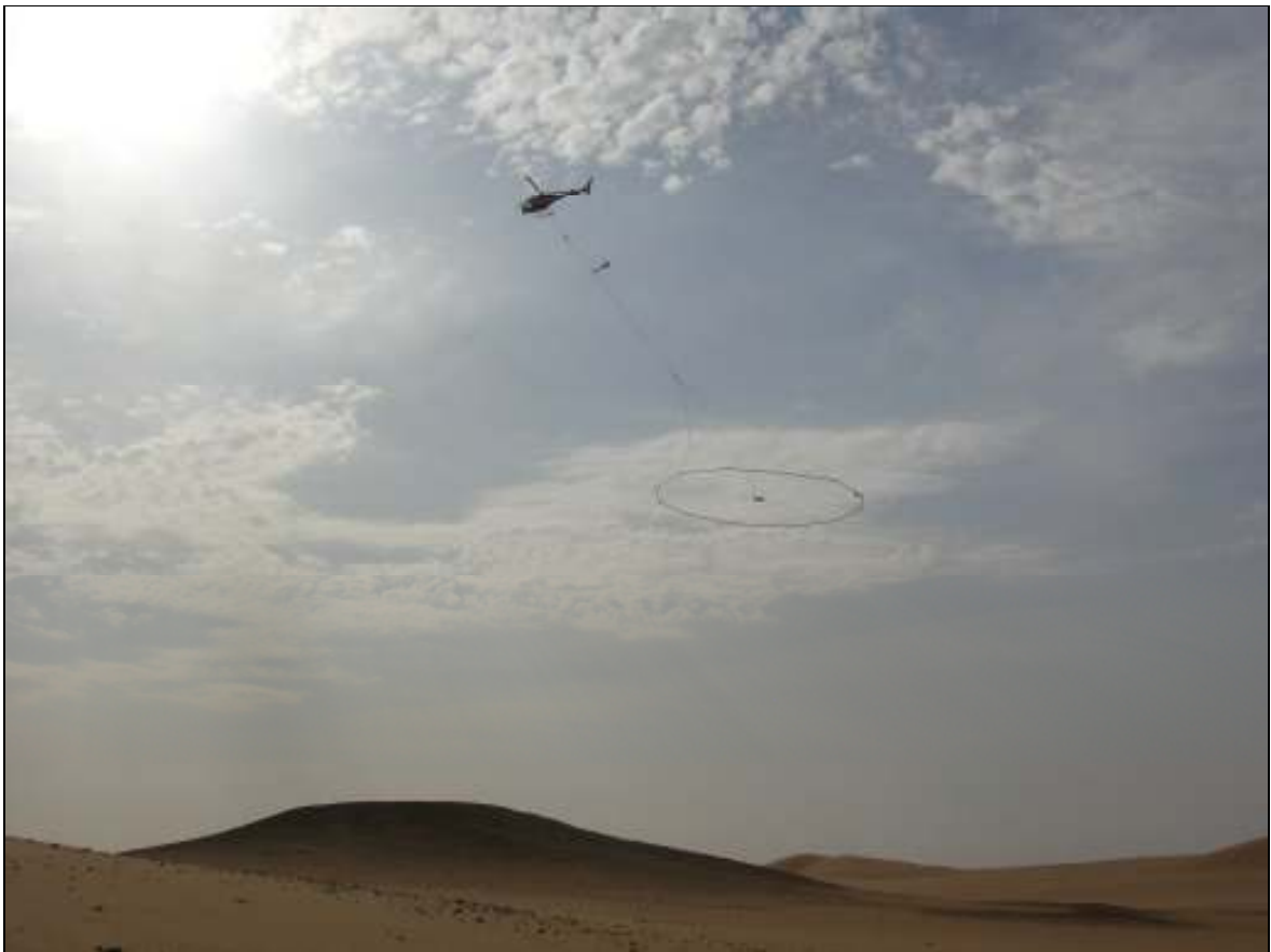
Picture – Example photograph of helicopter towing the VTEM geophysical sensor equipment
