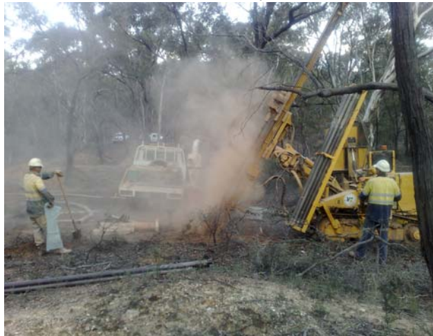
Collaring a hole at Wedderburn
