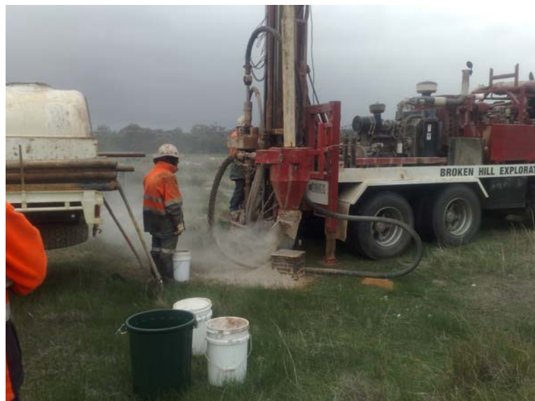
Aircore Drilling at Percydale
