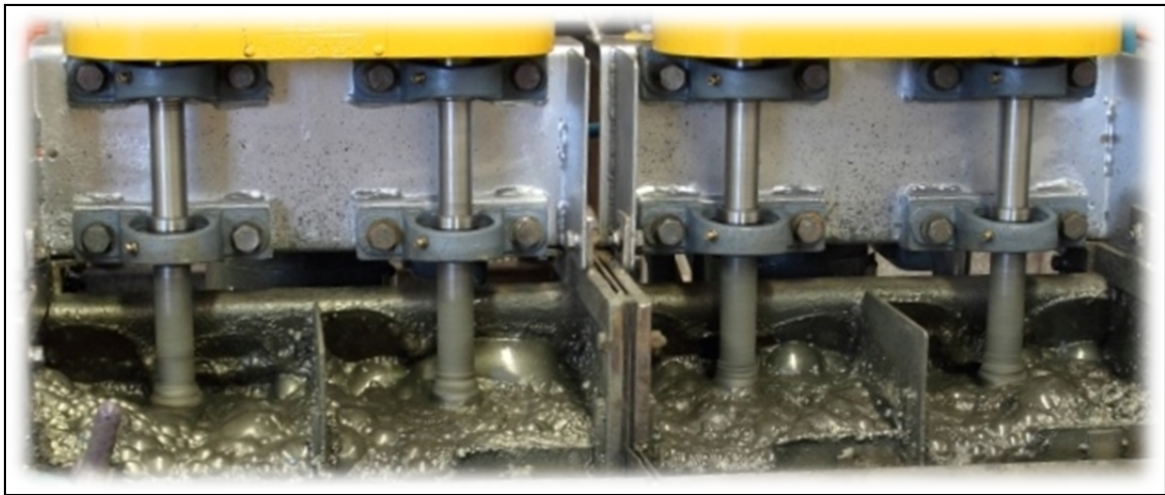
Figure 1: Copper-gold concentrate exiting floatation cell
