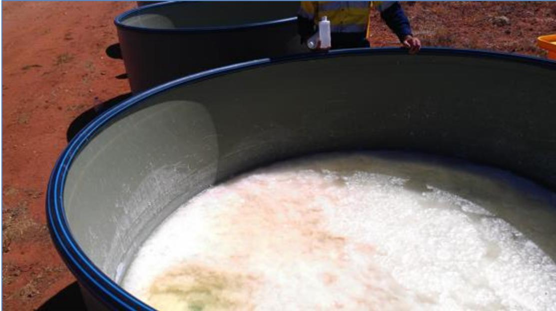
**Figure 2. Recent picture at Karinga highlights the amount of salt and potassic-rich bittern remaining after months of evaporation in a single tank. The bittern is now removed so that it may be crystallised for processing of potassium magnesium sulfate and other compounds.**
