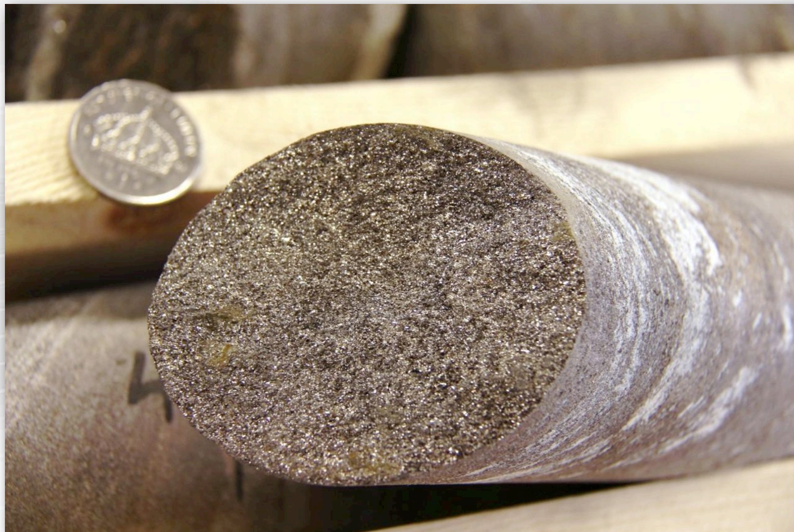
Talga drillcore at Raitajärvi, Feb 2013 showing coarse flake graphite.
