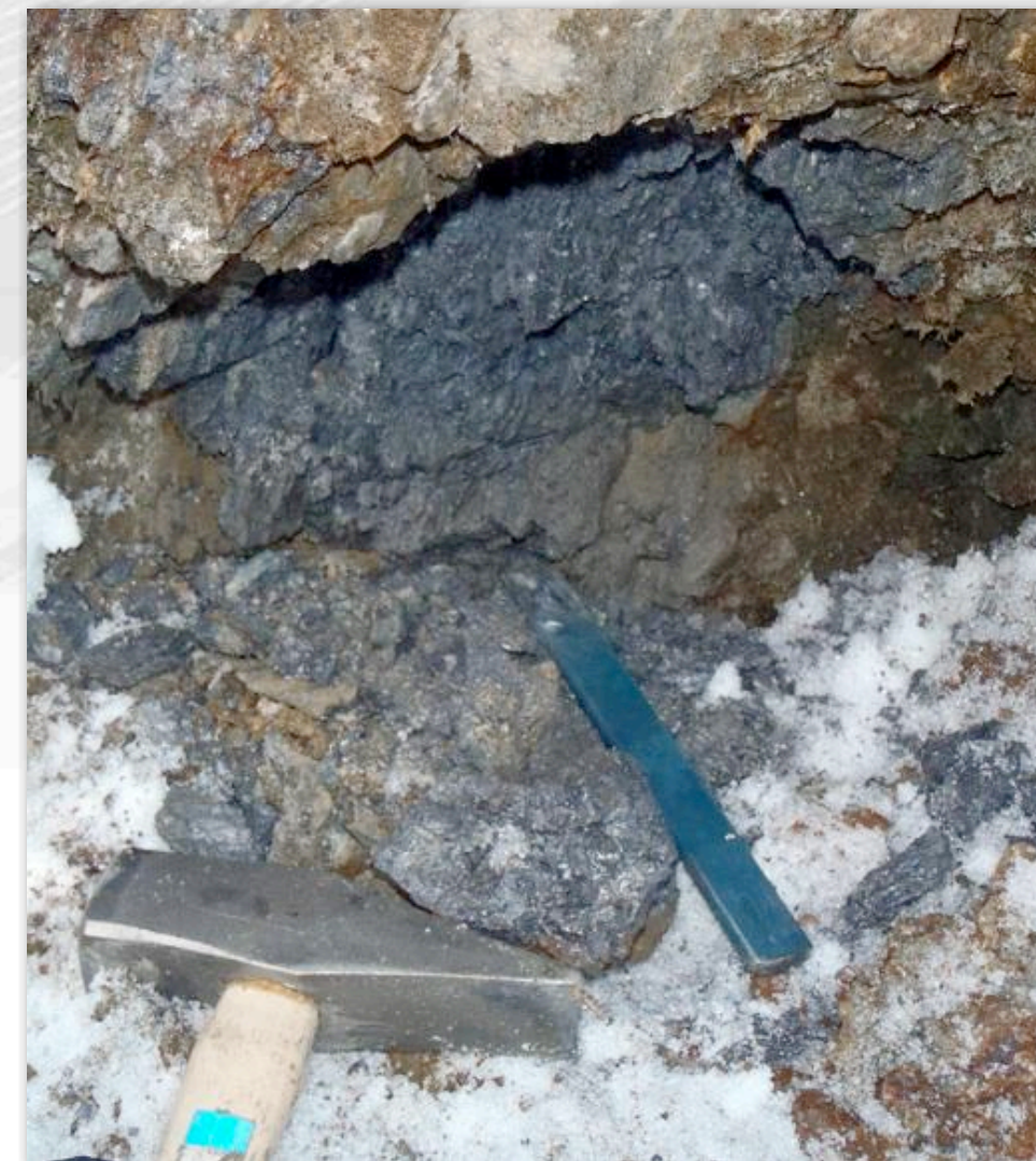
Coarse flake graphite in surface trench
