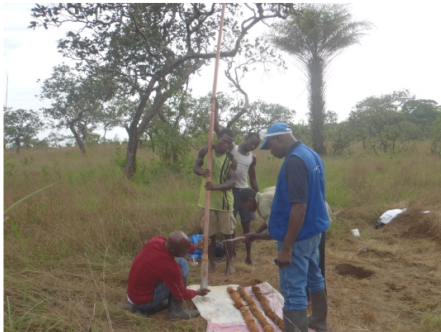
Hand auger drilling underway (left); recovered sample (right)
