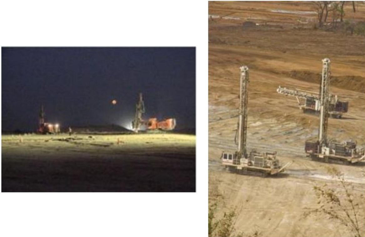
Figure 16.3 Drilling Blastholes in the Sabodala Pit
