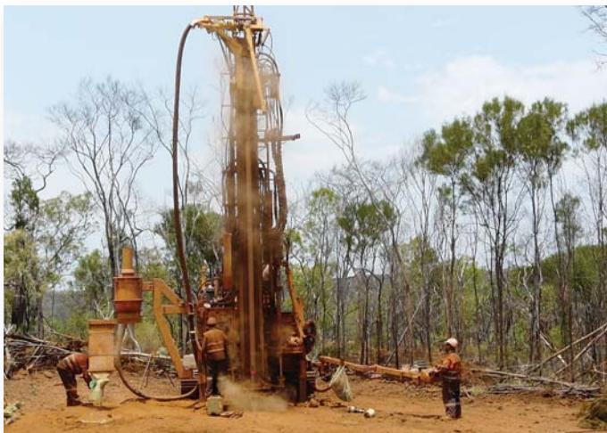
Mountain Creek project – Reverse Circulation drill rig.
