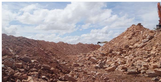
Stockpiled crusher feed material for concrete aggregate
