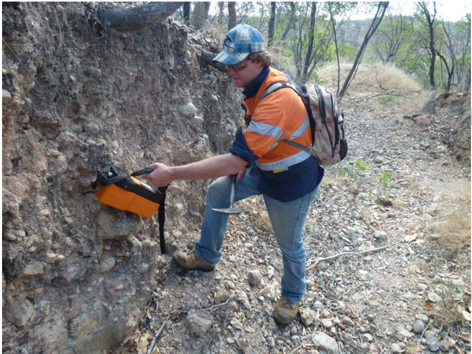
Uranium detection using a differential spectrometer
