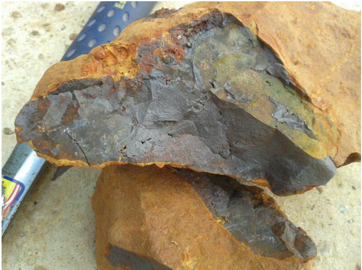
Photo: A sample of the hematite mineralisation from the first research pit delivered to Cabral's Brumado exploration office
