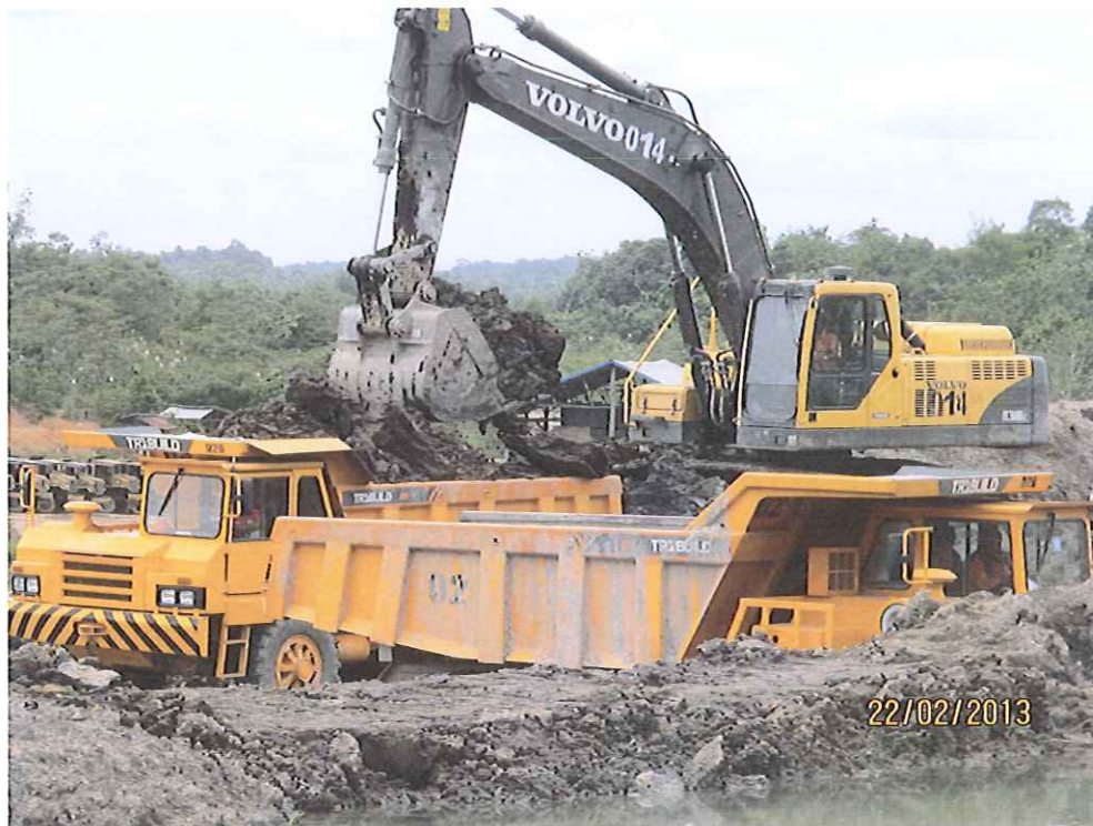
Figure 1: Photograph showing stripping of overburden in progress.
