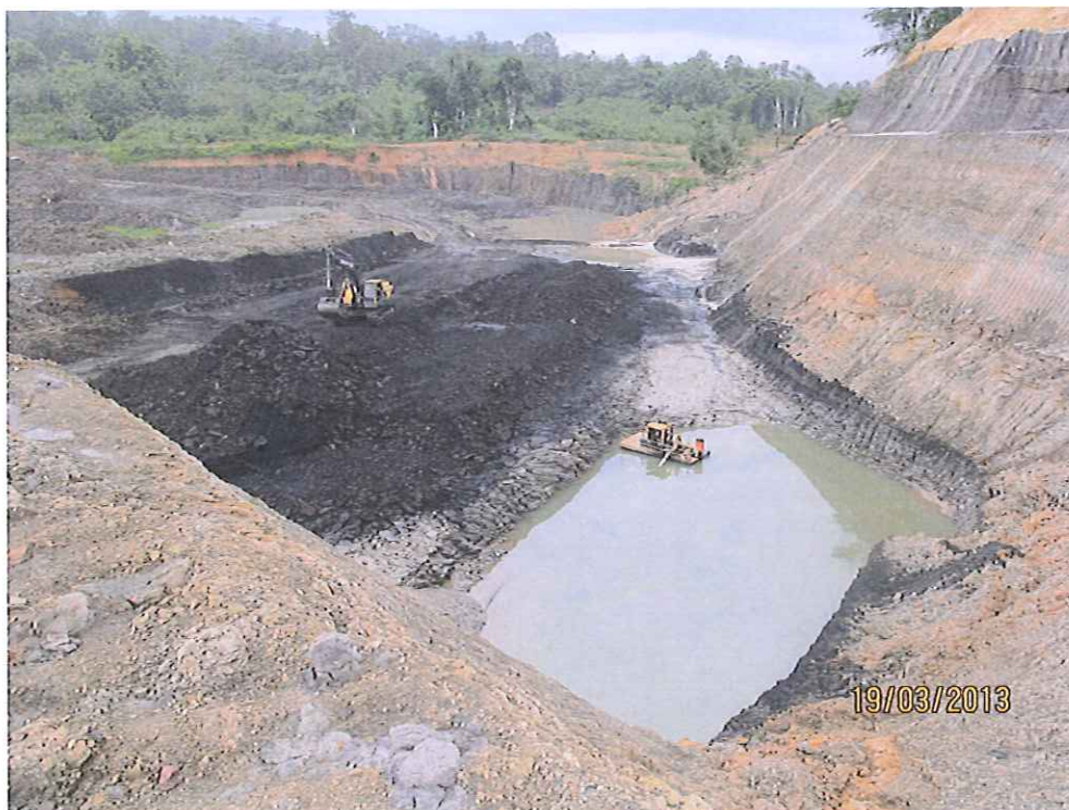
Figure 3: Photograph showing coal exposed in Seam B being prepared for extraction. At a higher elevation on the right is Seam A.
