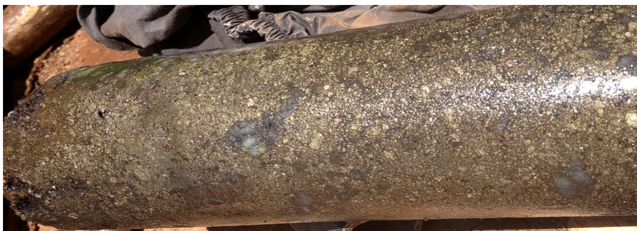
Figure 74: Example of high-grade drill core intersected in DODDH448 at Fairfield at approximately 83.2m which assayed 7.95% CuEq over 1m. Massive and semi-massive chalcopyrite and pyrite and minor chalcocite and bornite. Chalcocite contains 79.9% copper metal, chalcopyrite contains 34.6% copper metal, bornite contains 63.3% copper metal. Cobalt is associated with pyrite at Fairfield.
