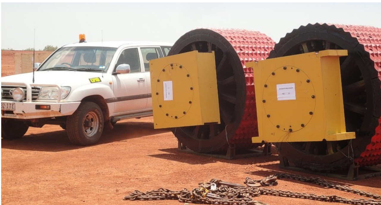
Figure 47: Rolls crusher fitted with specially designed replaceable face plates. In the native copper circuit 2 crushers are placed in series; the first processes 350 tonnes per hour and is powered by 2 x 280kW electric motors and the second processes 150 tonnes per hour and powered by 2 x 220 kW electric motors.
