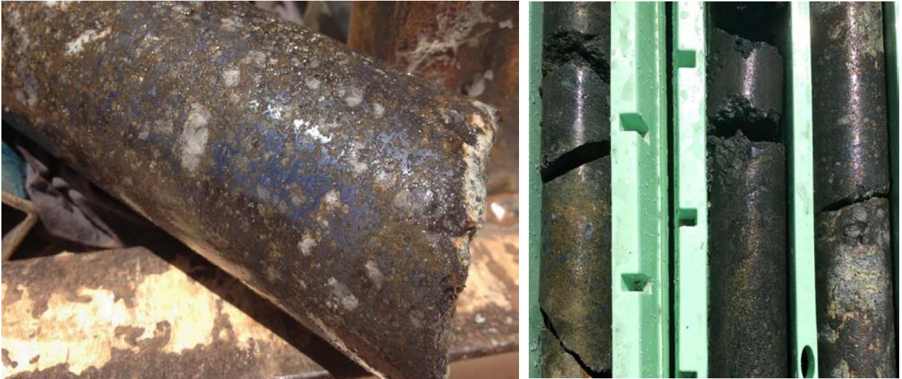
Figure 78: Example of high-grade drill core intersected in DODDH448 at Fairfield. Massive and semi-massive chalcocite (chalcocite contains 79.9% copper metal), and minor chalcopyrite (chalcopyrite contains 34.6% copper metal), bornite (bornite contains 63.3% copper metal) and pyrite (cobalt is associated with pyrite at Fairfield). Left approx. 83m, right approx. 81-84m
