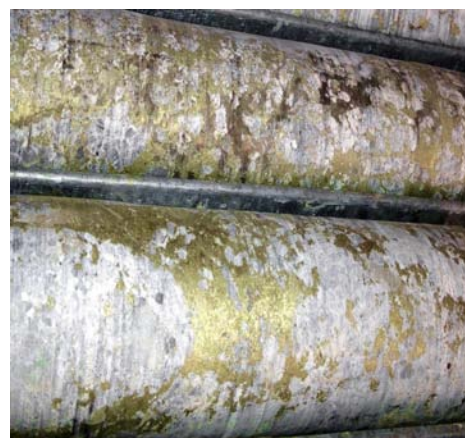
Figure 3: Diamond Drill core DODH456 showing semi-massive chalcopyrite in calcite/quartz breccia from approximately 160-162m that returned assay results of 7.66% Cu - chalcopyrite (34.6% copper metal)
