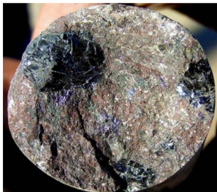
Figure 63: Pitchblende (uranium mineral), in diamond drill hole WUDH002.
