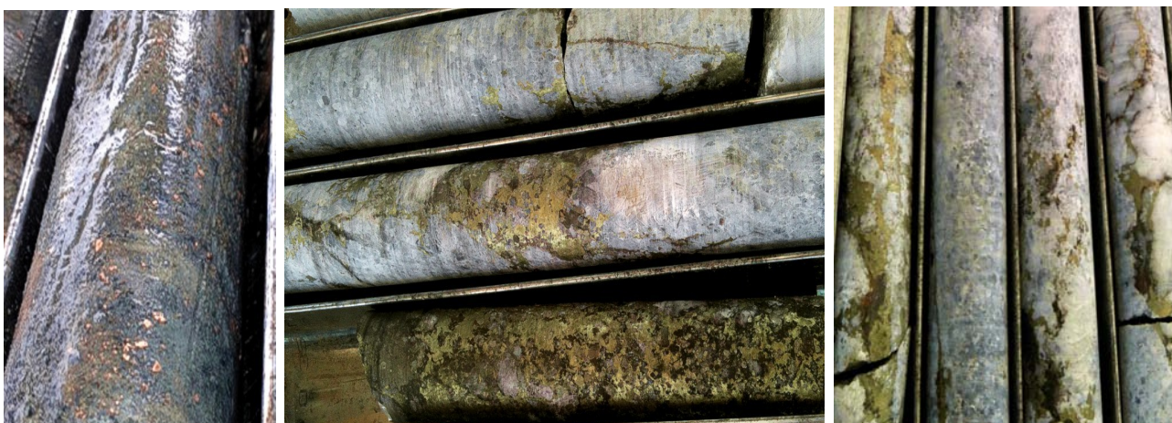
Figure 51: Diamond Drill core DODH457, left to right; native copper and chalcocite at approximately 33m and massive to semi-massive chalcopyrite from approximately 186-188m and 179-182m - chalcopyrite (34.6% copper metal) chalcocite (79.9% copper metal)
