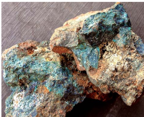
Figure 83: Sample of high-grade copper mineralisation taken from outcrop uncovered during earthworks; Malachite, azurite, chalcocite, chalcopyrite, bornite and fine-grain native copper within silicified siltstone breccia and magnetite.
