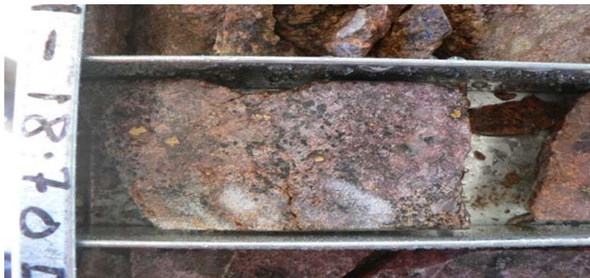
Figure 64: Carnotite (yellow uranium mineral), in diamond drill hole DODH248.
