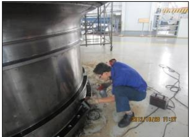
Figure 43: Finishing touches to Ball Mill bearing mount.
