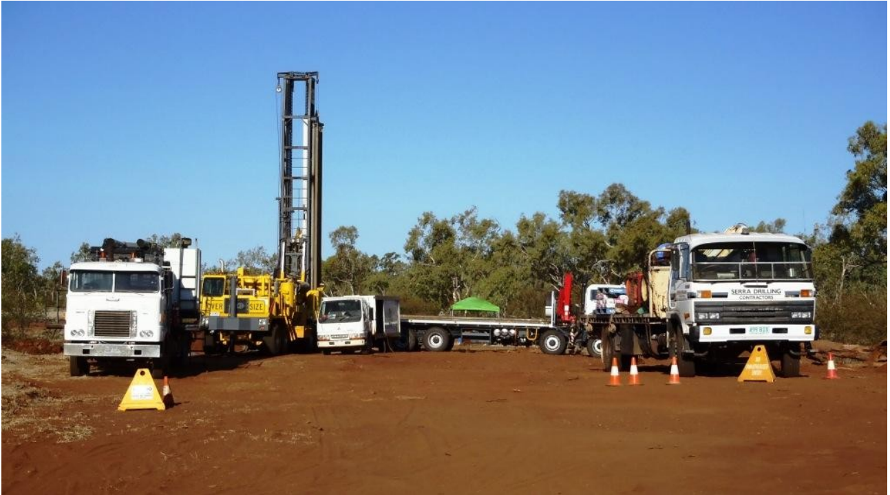
Figure 49: Pit dewatering activities (borehole drilling) - once completed, pumps divert the water to temporary storage facilities distributed throughout Rocklands for use in development works and will eventually be pumped to the WSF once it has been completed.
