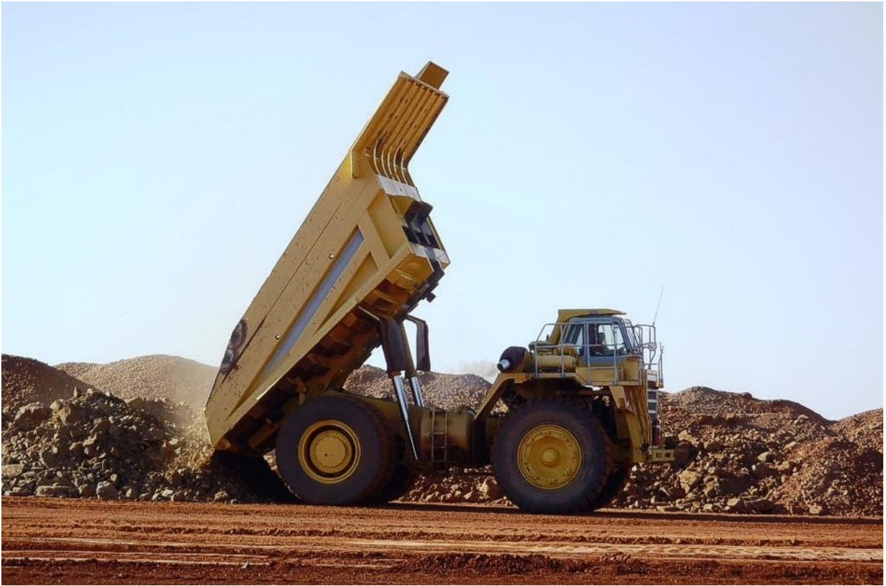
Figure 30: Dump truck unloads rock for use in the Water Storage Facility (WSF) Dam Wall construction.
