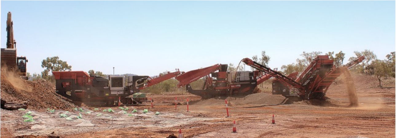
Figure 24: Mobile crushing circuit - rock suitable for road base and concrete construction is readily available at site.
