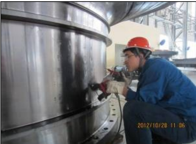
Figure 42: Finishing touches to Ball Mill bearing mount.
