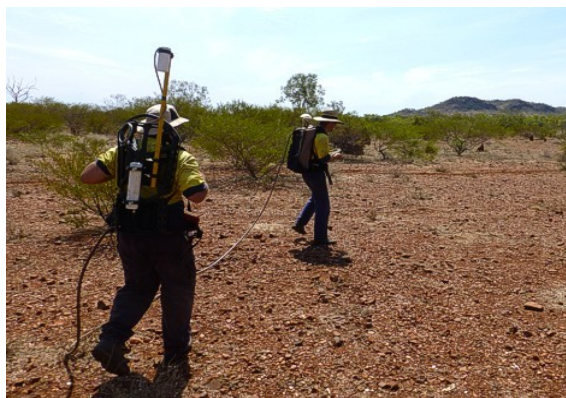
Figure 71: Readings being taken on survey-lines during the recent SAM surveys at Rocklands
