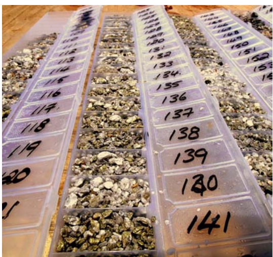
Figure 52: Metre after metre of high grade copper mineralisation intersected in wide-diameter pit-dewatering drill hole NVB038 - chalcopyrite (34.6% Cu metal) chalcocite (79.9% Cu metal) bornite (63.3% Cu metal) in hydrothermal breccia (assays awaited)
