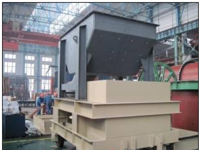
Figure 45: Ball Mill product discard collection sump and chute
