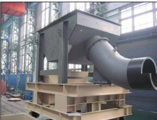
Figure 44: Ball Mill product discard collection sump and chute
