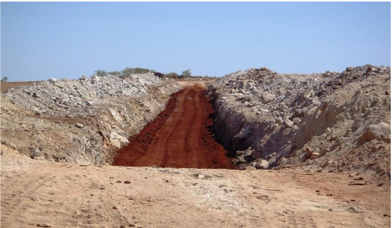
Figure 33: The iron-rich clays are easily distinguished from the light coloured (Corella Formation) rocks.
