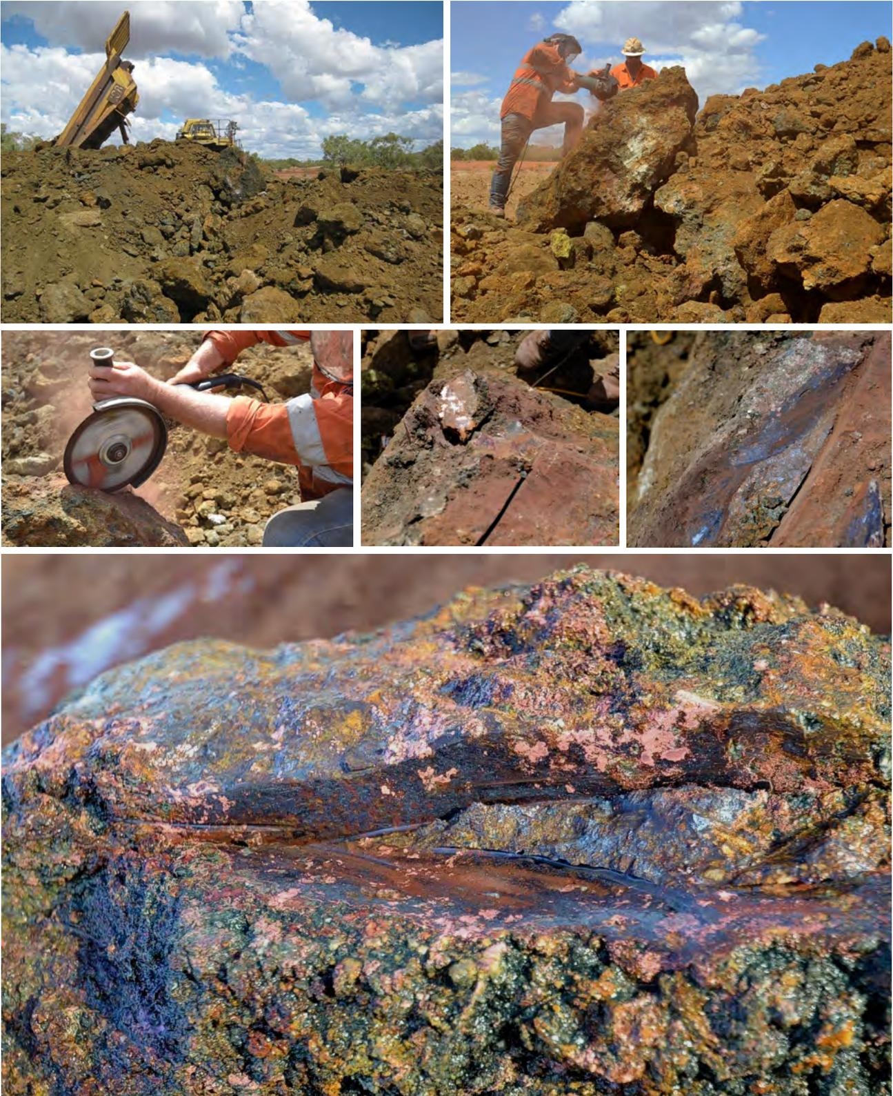
Figure 7: Native copper stockpile - in sequence diamond saw cutting of small sample wedge from large boulder that was visually "unexciting" but found to contain significant copper including native copper (99.65% copper), cuprite (88.8% copper) and chalcocite (79.85% copper).
