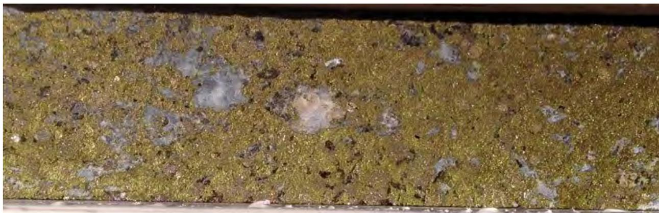
Figure 5: Diamond drill core DODH472 (wet core) showing semi-massive to massive chalcopyrite and pyrite in calcite/quartz breccia from approximately 188.5m to 189.5m - chalcopyrite contains 34.6% copper metal and pyrite is typically associated with cobalt at Rocklands. Hole is currently drilling ahead in mineralisation.
