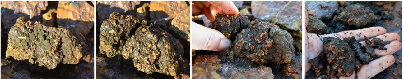
Figure 17: Solid clay with visible native copper after passing through the crushing circuit (left), begins to break up under its own weight as water is added (centre) and can be easily broken by hand as the clays dissolve after just a few minutes of soaking (right).
