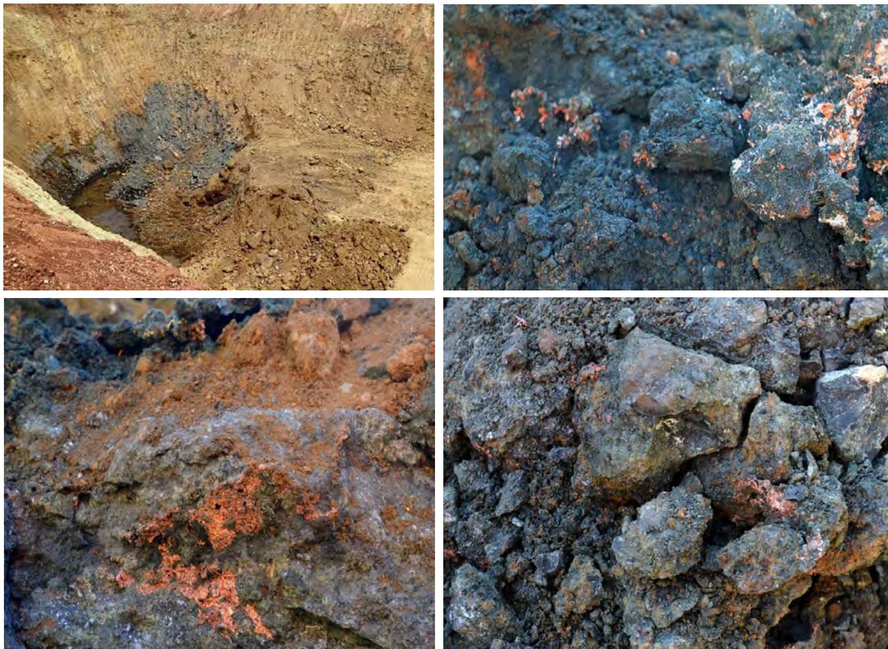
*Figure 14: Left; final depth of box-cut excavation showing the top of the exposed coarse native copper zone in a mixture of clays and fresh-rock and right; close up of the easily distinguishable blue-grey native copper ore.*
