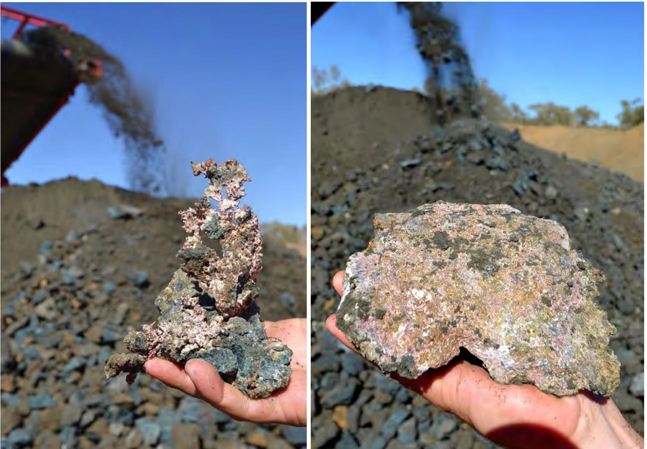
Figure 18: Examples of native copper masses being liberated in the first-stage of test-crushing through the Company's mobile crushing circuit...chalcocite ore also rich in native copper can be seen in the background. It appears a DSO concentrate of 20% Cu or more will be possible that includes both chalcocite and native copper species. The DSO will also include cobalt, gold and magnetite credits.
