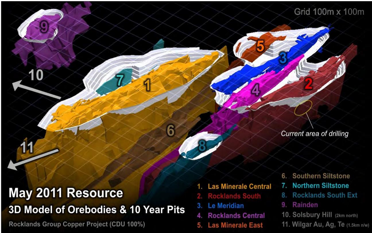
Figure 44: 3D rendered model showing main Rocklands Orebodies and 10-year Final Pit Designs (Rocklands South is to the right)
