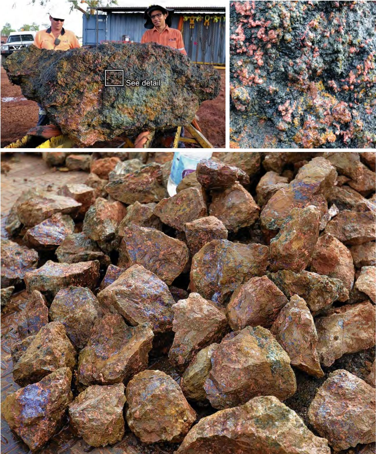
Figure 19: Top left; large 3 tonne agglomerated mass of native copper and top right; close-up of detailed area. Main image; Remains after being crushed through the coarse screen (<120mm) of the mobile crushing circuit. The sample is estimated to contain 40% Cu from a combination of copper species including native copper (99.65% Cu), cuprite (88.8% Cu), and chalcocite (79.85% Cu), +/- tenorite, malachite, azurite and minor chalcocopyrite.
