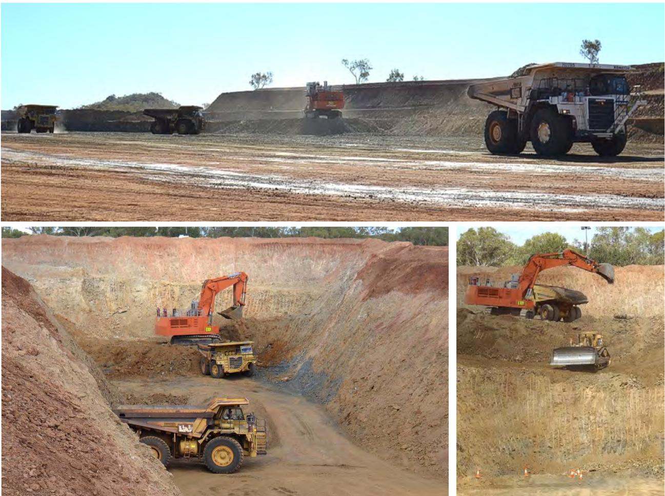
Figure 11: Top image; Las Minerale pit taking shape as the entire pit area is excavated to a single working bench level (RL215m). Bottom images; 20m deep box-cut excavation in the middle of Las Minerale (reached RL195)
