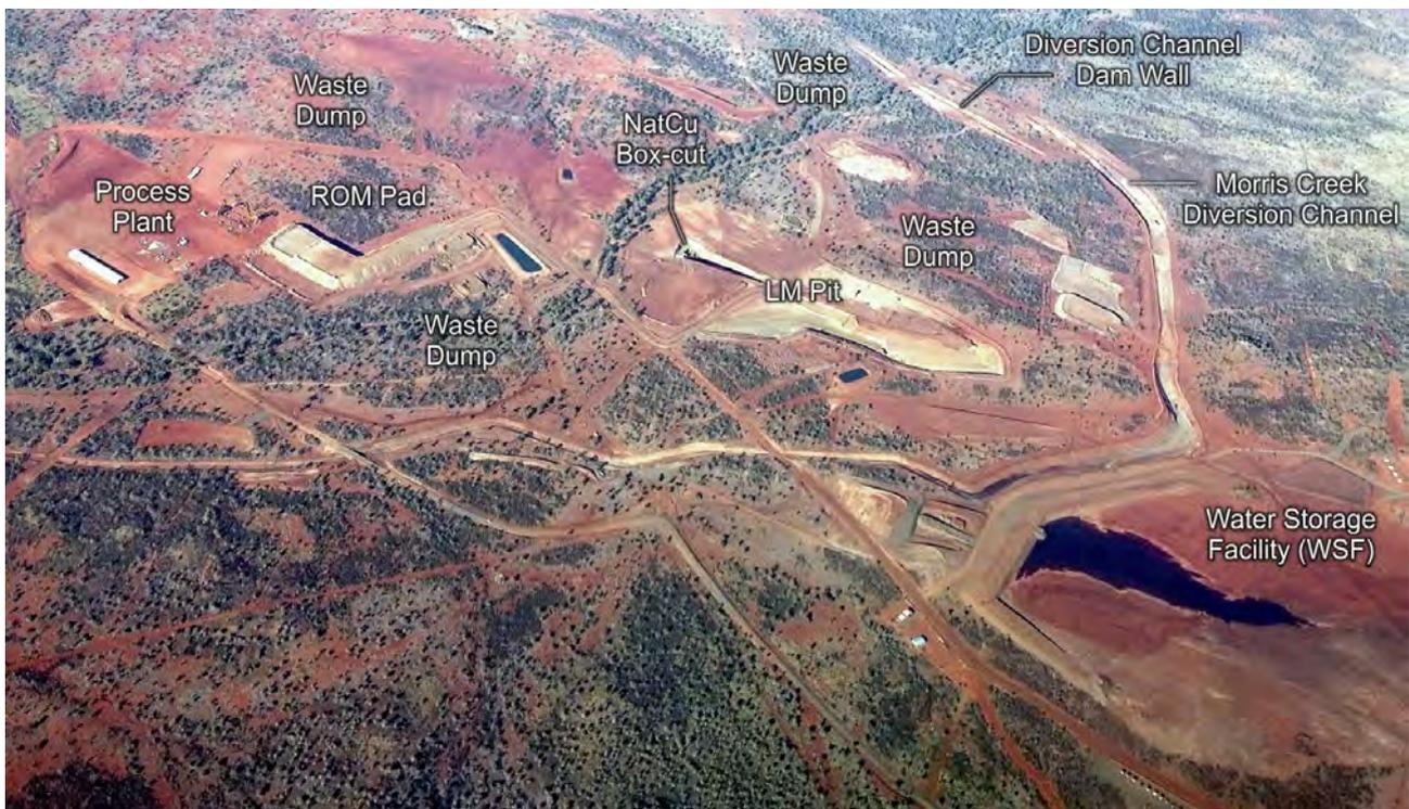
Figure 20: Aerial photo of the main development areas at Rocklands, showing the Las Minerale pit outline taking shape (LM Pit), and location of recently excavated small box-cut (NatCu Box-cut) in the centre of Las Minerale, to obtain coarse native copper ore for commissioning of the crushing circuit.
