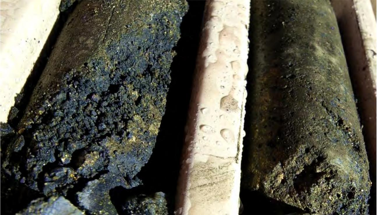
Figure 38: Diamond drill core DODH465 showing supergene copper mineralisation from approx. 245-246m which assayed 10.4% Cu.
