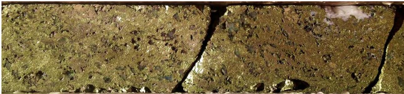
Figure 4: Diamond drill core DODH472 (wet core) showing massive chalcopyrite and pyrite in calcite/quartz breccia at approximately 187m - chalcopyrite contains 34.6% copper metal and pyrite is typically associated with cobalt at Rocklands. Hole is currently drilling ahead in mineralisation.
