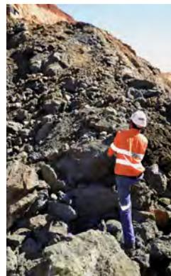
Figure 9: High-grade chalcocite suitable for Direct Shipping Ore (DSO) being excavated from the base of the Las Minerale Starter Pit, with estimated grades ranging from 20-60% copper, based on visual estimates, confirmed with XRF analysis. Image of XRF showing 54.7% Cu result from the face of a large chalcocite boulder.
