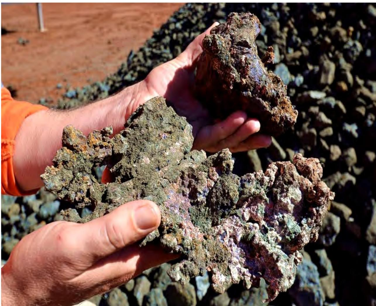
*Figure 15: Examples of native copper masses being liberated during test-crushing through the Company's mobile crushing circuit...chalcocite ore (blue-grey) also rich in native copper can be seen in the background. It appears a DSO concentrate of 20% Cu or more will be possible that includes both chalcocite and native copper species. The DSO will also include cobalt, gold and magnetite credits.*
