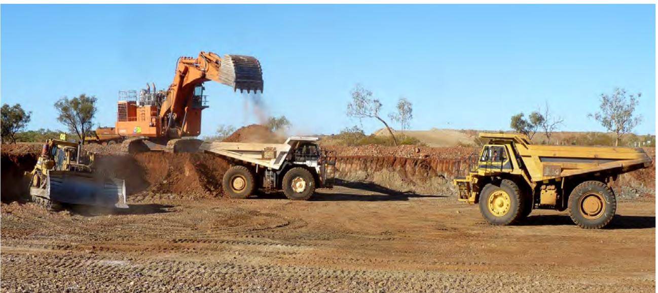
*Figure 32: Excavation starts at the eastern end of the Las Minerale Pit (LM Pit), which is being excavated down to the same level as the northern end of the Pit (RL 215), to create a single working platform. The ROM pad can be seen in the background.*
