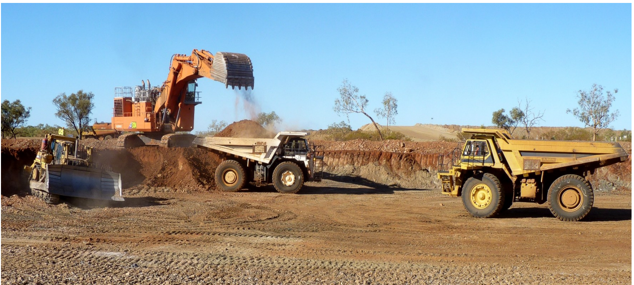
Figure 14: Excavation starts at the eastern end of the Las Minerale Pit (LM Pit), which is being excavated down to the same level as the northern end of the Pit (RL 215), to create a single working platform. The ROM pad can be seen in the background.
