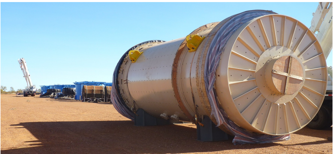
Figure 10: Native Copper Cleaning Drum delivered to lay-down area (Flotation Cells in background)
