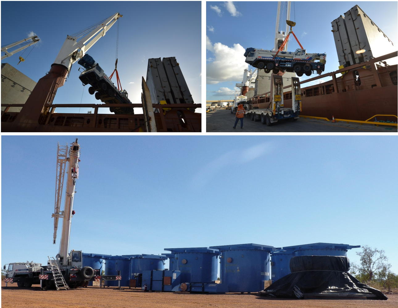
Figure 4: Delivery of large crane at the Port of Townsville (top) to be used at the Rocklands Process Plant site, pictured (above) with Flotation Cells and end-cap for Ball Mill.
