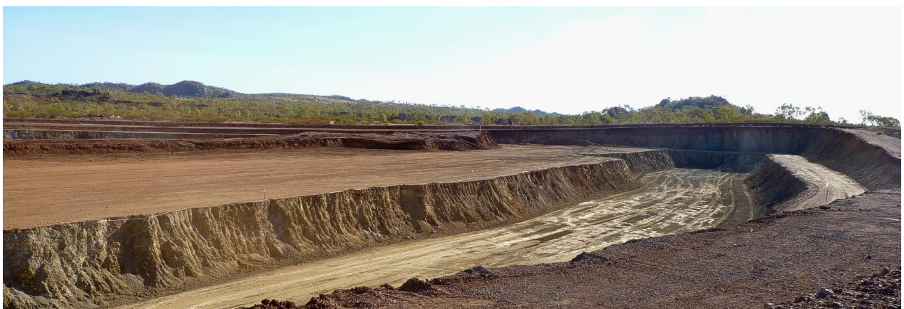
Figure 13: North-west end of Las Minerale Pit, showing ore-zones left in centre of pit and waste areas either side being removed for use in various infrastructure requirements.
