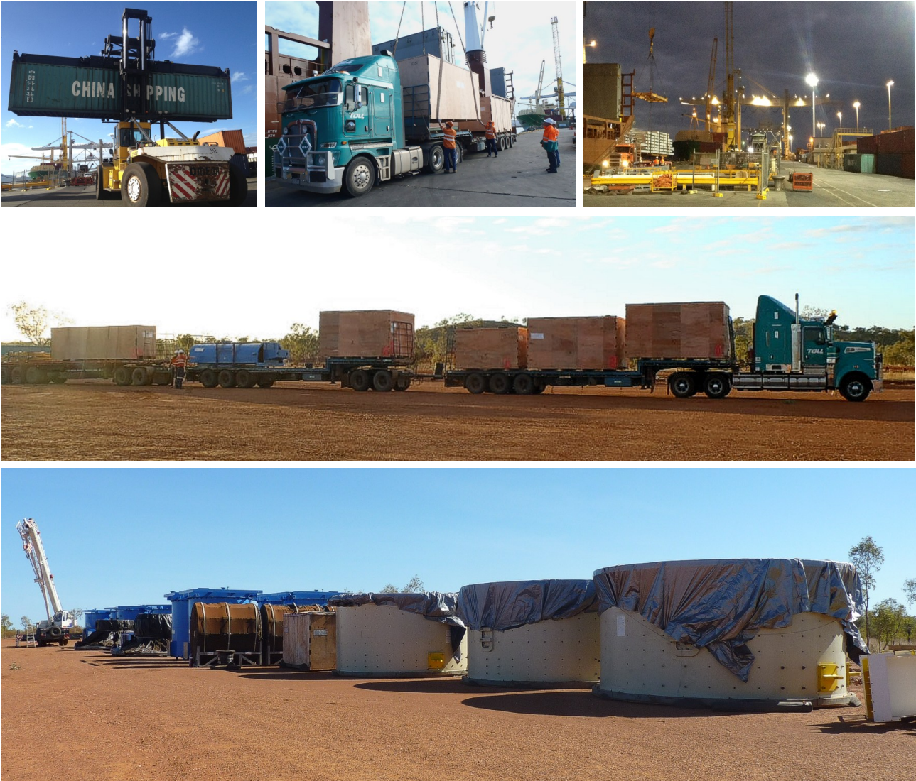
Figure 5: Various components continue to be shipped to the Port of Townsville (above), delivered to site via road-train (middle), and set-down for assembly as/when required (below) at the Process Plant site.
