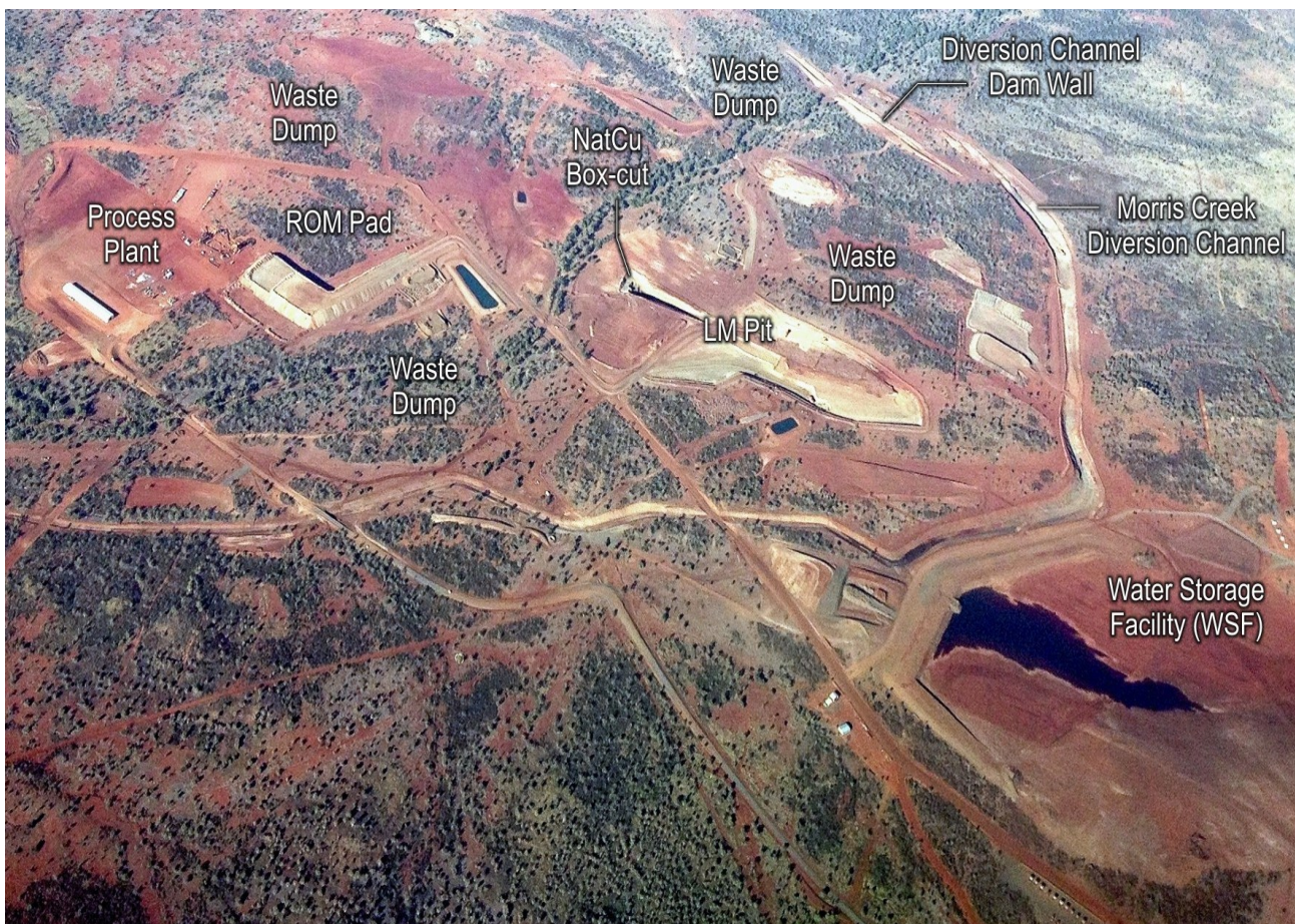
Figure 1: Aerial photo of the main development areas at Rocklands, showing the Las Minerale pit outline taking shape (LM Pit), and location of recently excavated small box-cut (NatCu Box-cut) in the centre of Las Minerale, to obtain coarse native copper ore for commissioning of the crushing circuit.
