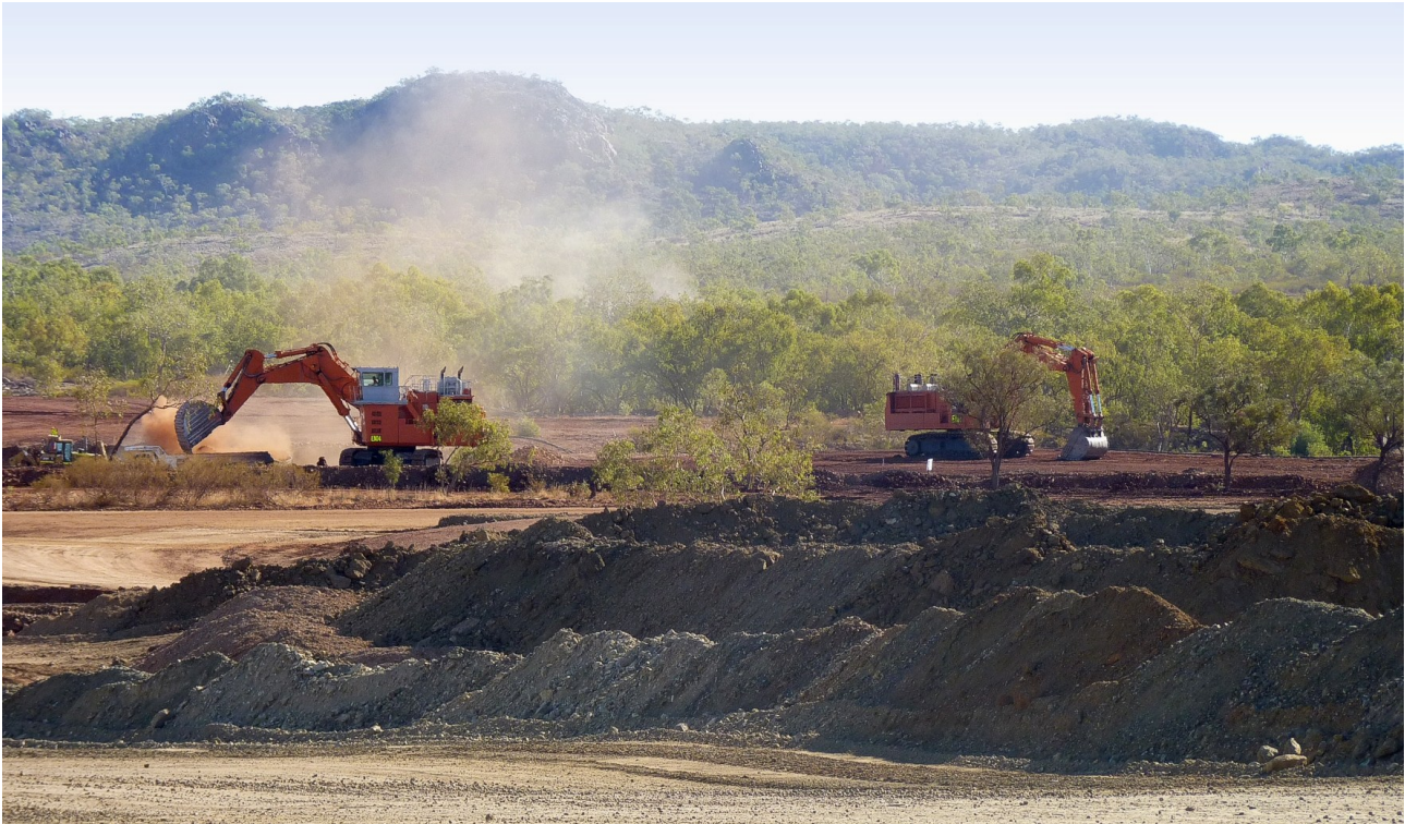
Figure 16: View from the ROM Pad looking towards the eastern end of the Las Minerale Pit, which has just started and will eventually be excavated to the same level (RL215) as the north-west end.
