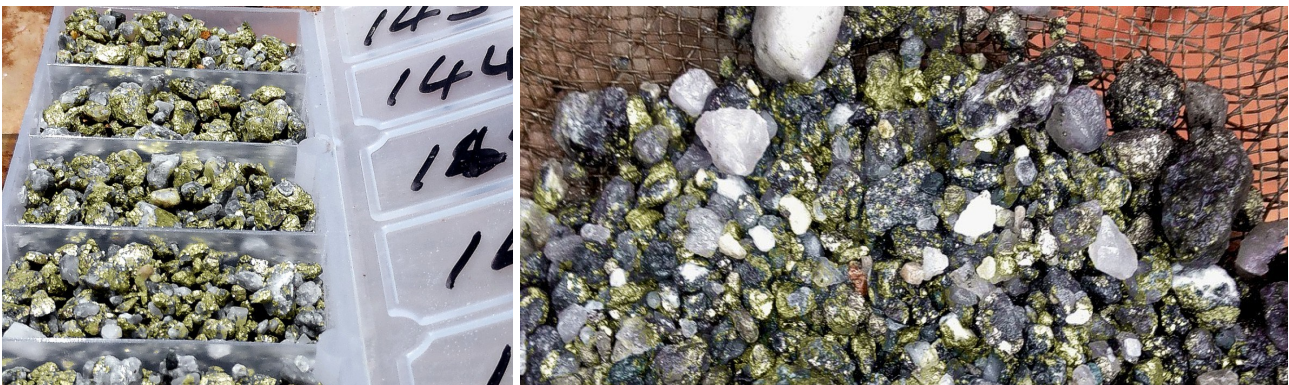
Figure 1: High grade copper mineralisation including chalcopyrite, chalcocite and bornite in drill chips from pit dewatering drill hole NVB038 from 143-146m (left) and NVB038 from approximately 107m (right) - chalcopyrite (34.6% copper metal) chalcocite (79.9% copper metal) bornite (63.3% copper metal) in hydrothermal breccia (assays awaited)
