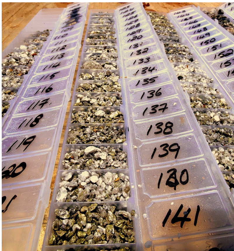
Figure 5: Metre after metre of high grade copper mineralisation intersected in wide-diameter pit-dewatering drill hole NVB038 - chalcopyrite (34.6% Cu metal) chalcocite (79.9% Cu metal) bornite (63.3% Cu metal) in hydrothermal breccia (assays awaited)
