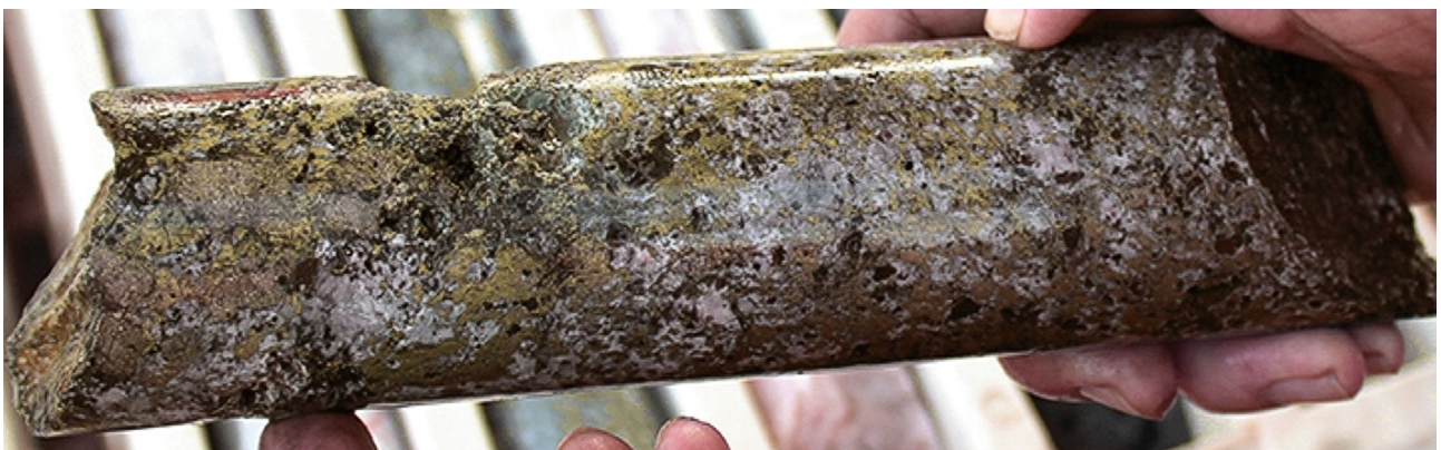
Figure 1: Diamond drill core DODH478 (wet core) showing semi-massive to massive sulphides including chalcopyrite (yellow), and pyrite (silver-grey) in calcite/quartz breccia from approximately 239m (12% visual chalcopyrite) chalcopyrite contains 34.6% copper metal and pyrite is typically associated with cobalt at Rocklands.
