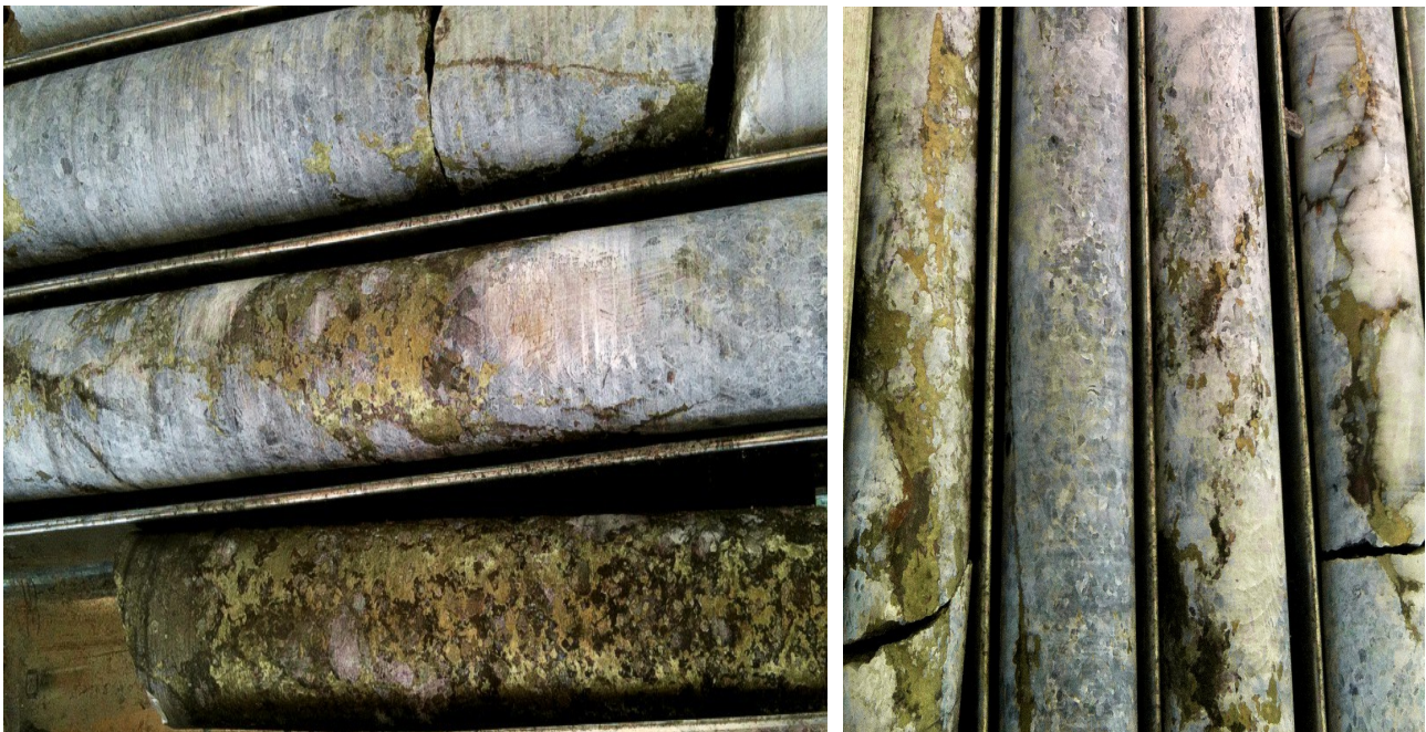
Figure 4: Diamond Drill core DODH457 - massive to semi-massive chalcopyrite from approximately 186-188m (left) and 179-182m (right) - chalcopyrite (34.6% copper metal) chalcocite (79.9% copper metal).
