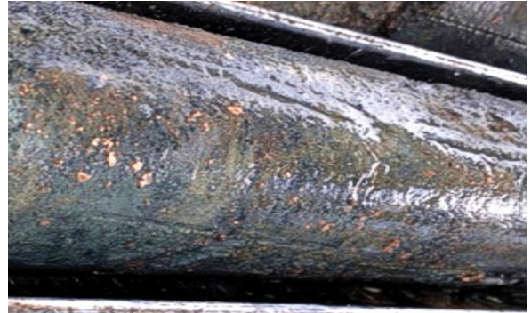
Figure 6: Native copper and chalcocite at approximately 33m in diamond drill hole DODH457. Native copper contains 99.8% copper metal and chalcocite contains 79.9% Cu metal..
