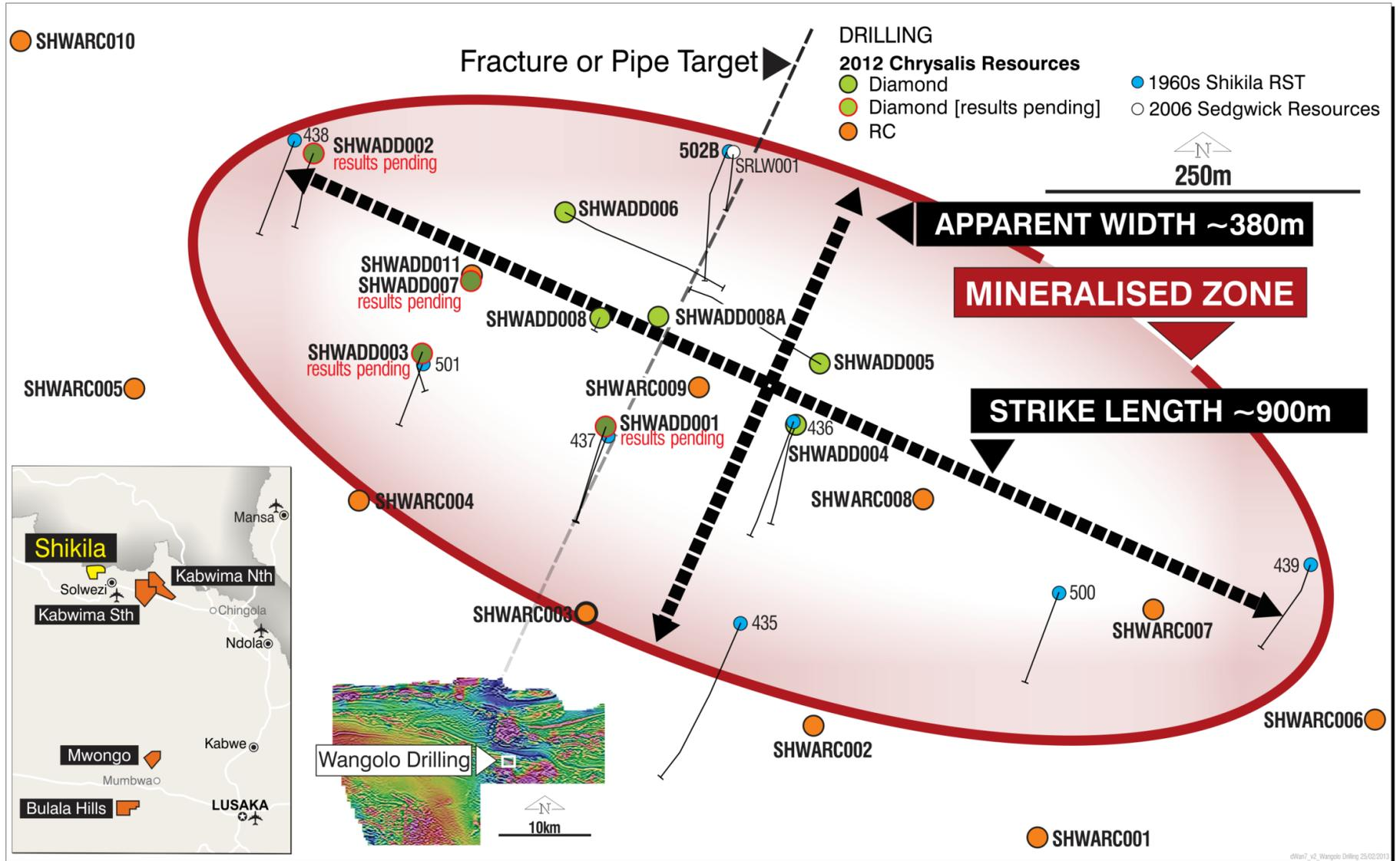
Figure 1: Drill hole locations and copper intersections for the RC and DD drilling at the Wangolo Prospect
