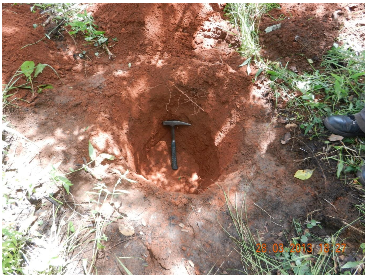
Pit at Kabwima Block G showing red residual soil
