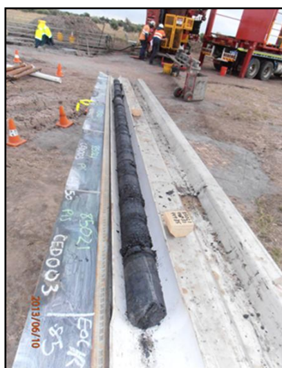
Core drilling samples from Pisces Seam at Mackenzie, June 2013
