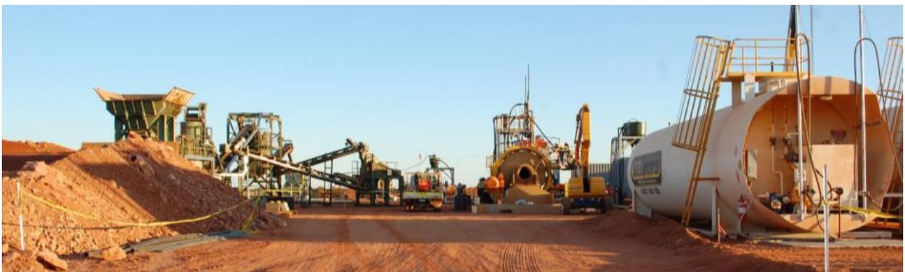
**Figure 4. Wide-angle photograph of Pilot Processing Facility. Crushing circuit on the left, ball mill centre right (with Knelson concentrator behind) and fuel tanks / generators on the right.**
