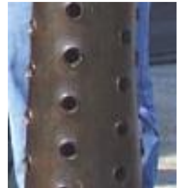
Perforated steel casing
