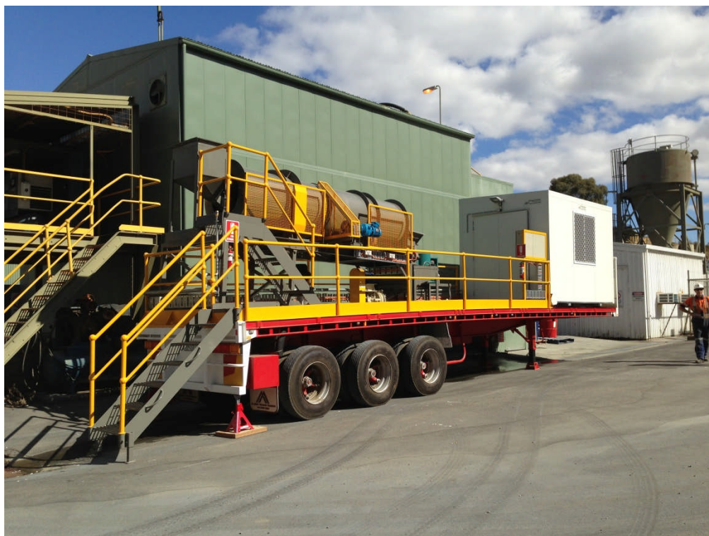
Figure 1: Gravity Circuit installed at Maldon treatment plant
