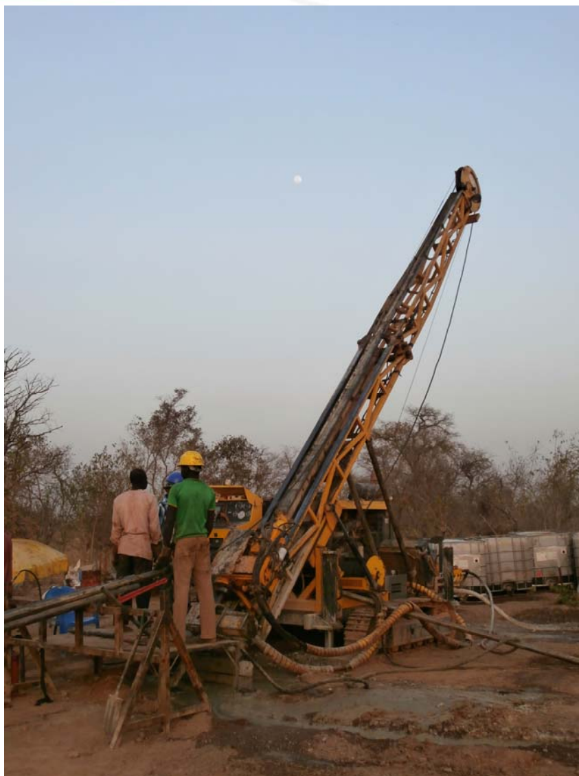
Figure 2: Photograph taken of Australian Mines' diamond core drilling operation at Yargarma. This drill hole (hole number YADD008 ) has a planned depth of 150 metres and is targeting a geophysical lineament that coincides with historic artisanal gold workings.
