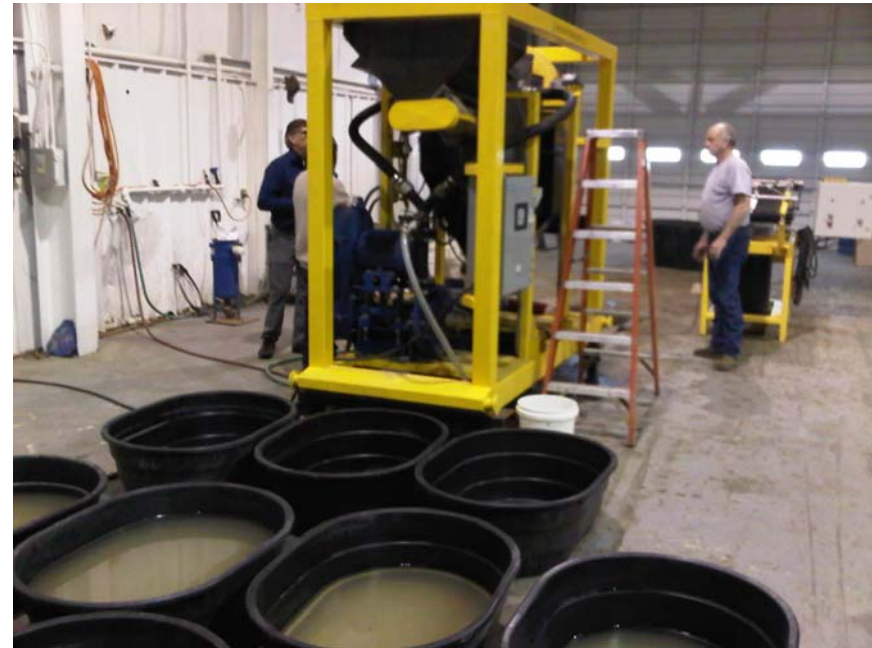
Pilot-scale Ablation unit that processes ~0.5 tonnes/hour in operation undertaking testwork. This technology is being scaled up to units that can process ~5 tonnes/hour.
