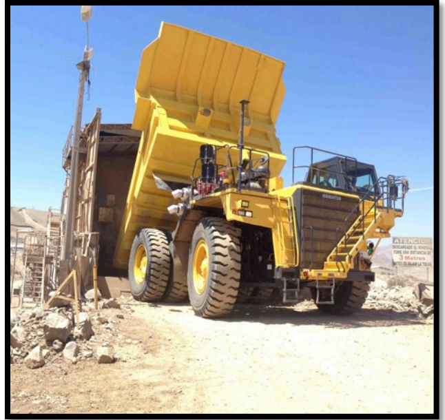
Figure 14 - Dumping into the Primary Crusher
