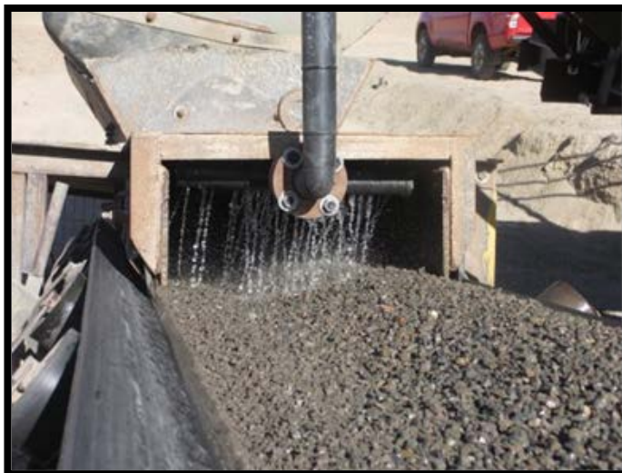
Figure 16 – Pre-cyanidation of crushed ore
