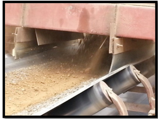
Figure 8 – Tailing added to crushed ore
