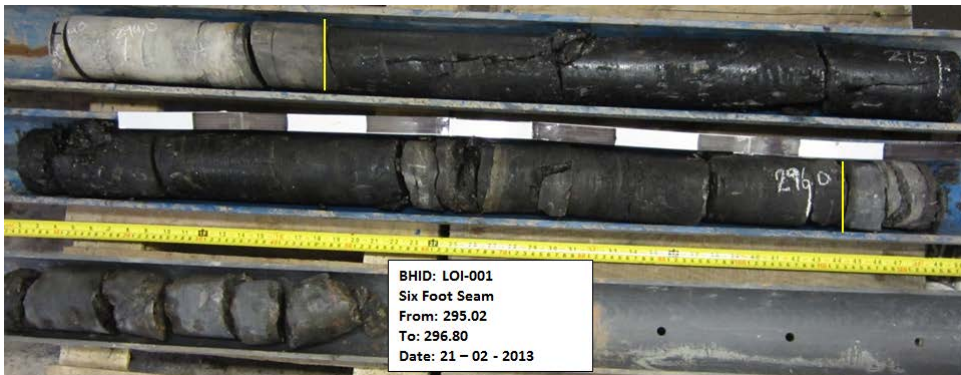
Figure 2: LOI-001 - Six Foot Coal Seam Core
