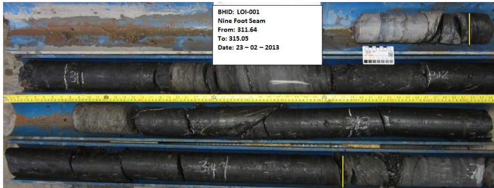
Figure 3: LOI-001 - Nine Foot Coal Seam Core 1
