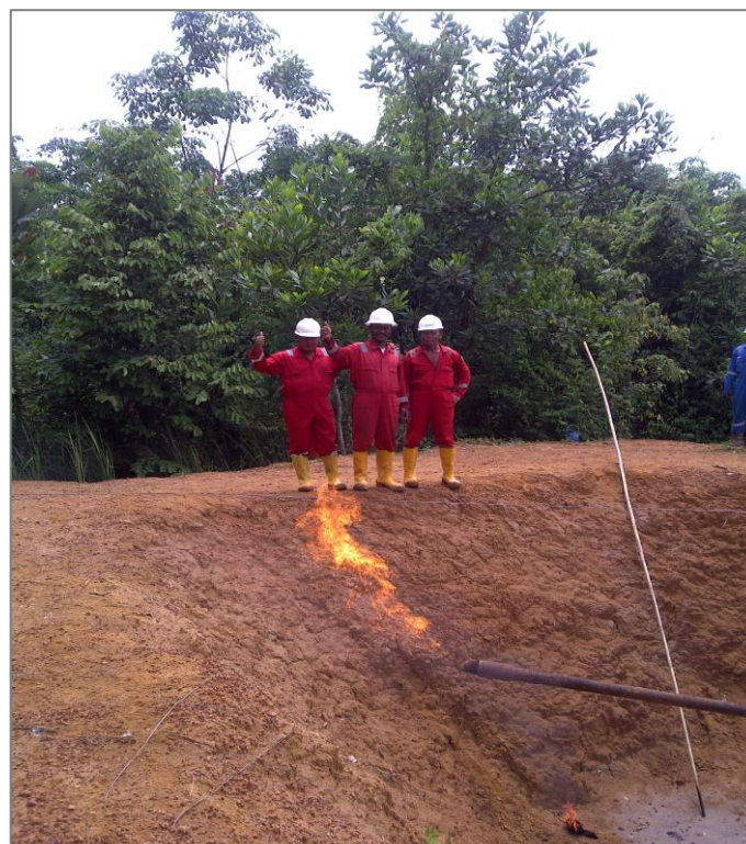
Image 1: First gas shows during Pilot Well #2 completion
