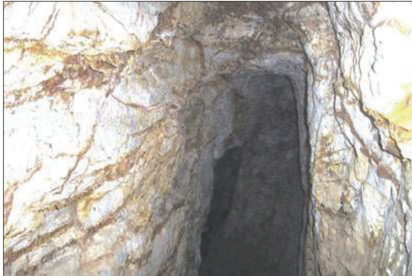
Figure 16: Crudine-Edwards Adit with quartz-limonite stockwork in sediments with Antimony-Gold Mineralisation.
