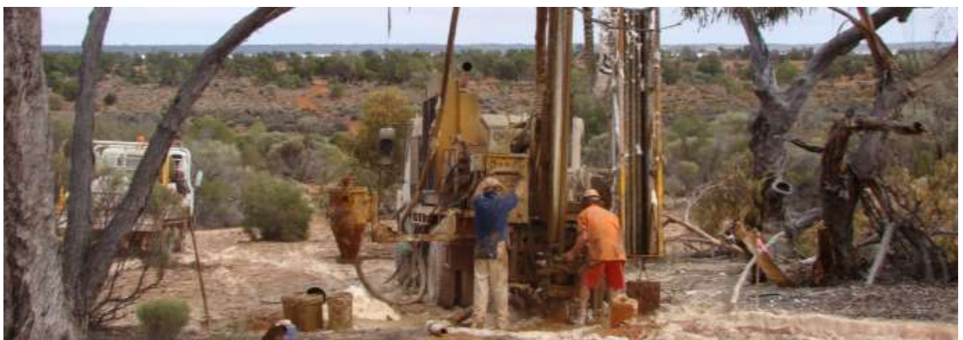
Aircore drilling at the Burns Prospect
