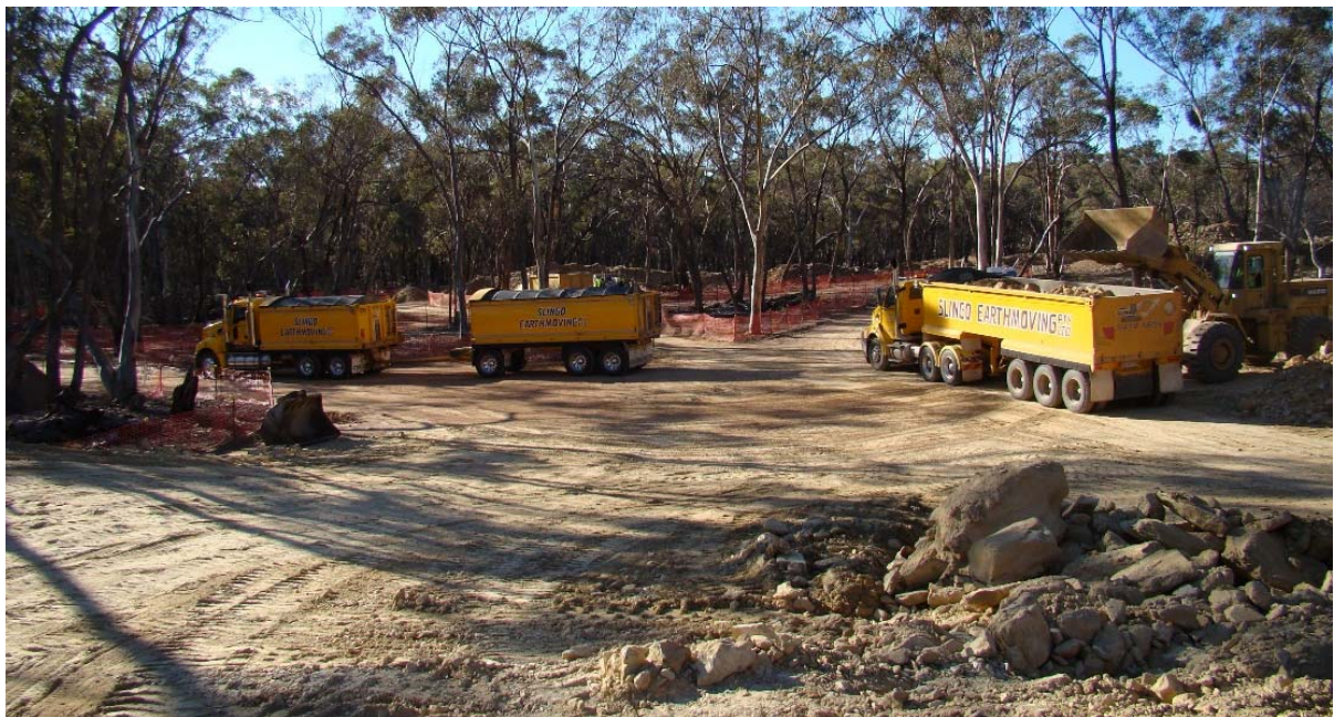
Figure 2. Example of ore being loaded onto road trucks (Black Reef Mine)
