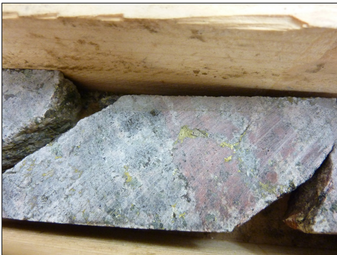
Figure 6. Copper and gold mineralisation in ALT11006; 3m @ 1.3% Cu, 5.2g/t Au from 15m
