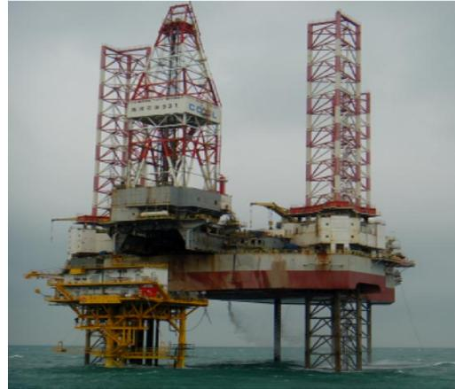
*HYSY 931 rig at WZ 6-12 wellhead platform for development drilling*
