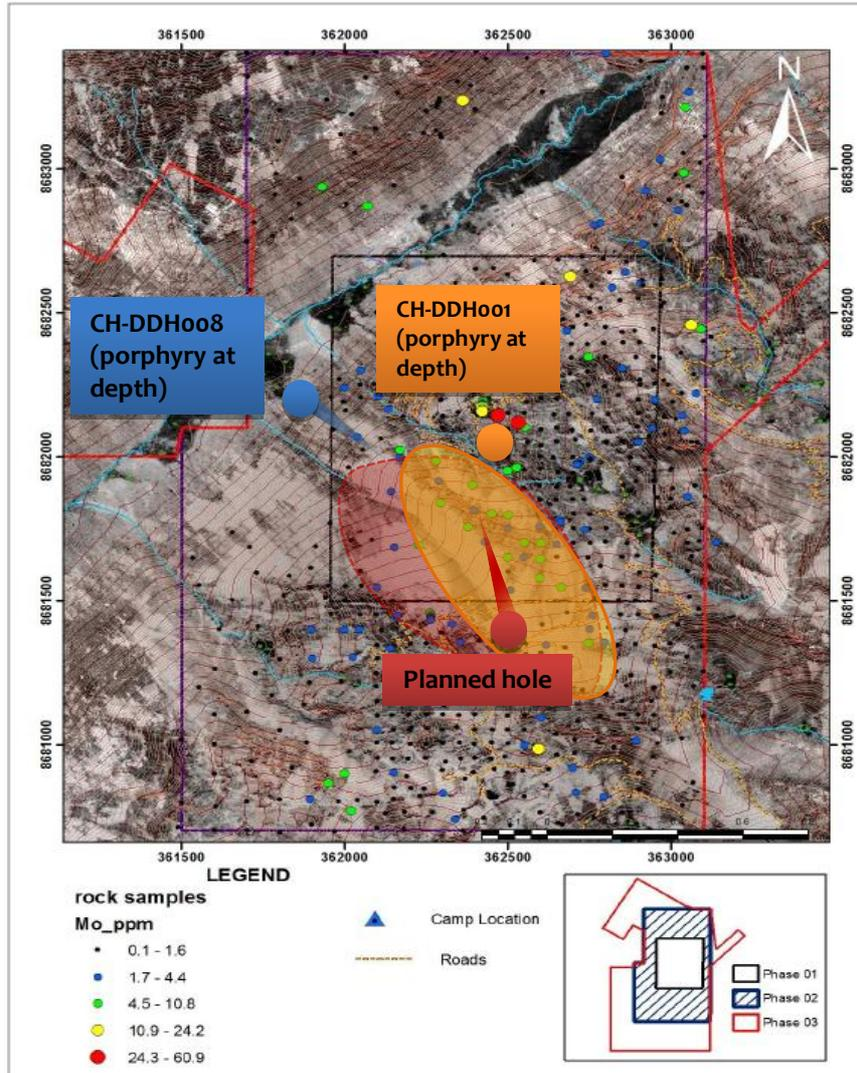
Figure 3: Coincident molybdenum geochemical anomaly (orange shaded area) and large argillic/phyllitic alteration anomaly (red shaded area) with CH-DDH001 and CH-DDH008.
